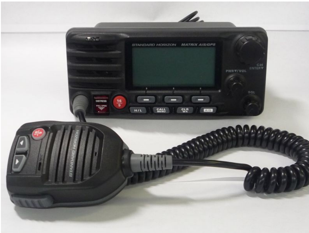
Front view and Microphone (GX2200) Built-in a GPS receiver circuits.
