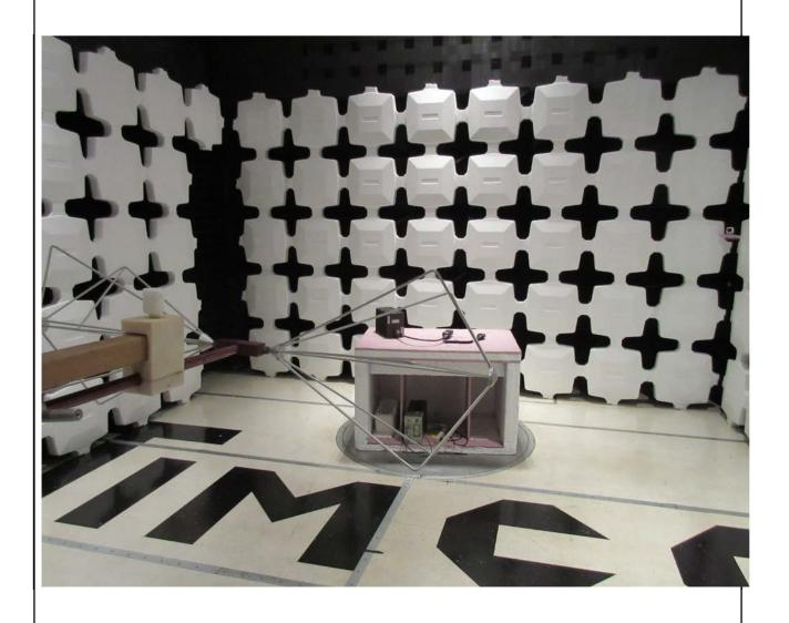
Field strength of spurious emissions (Radiated)
