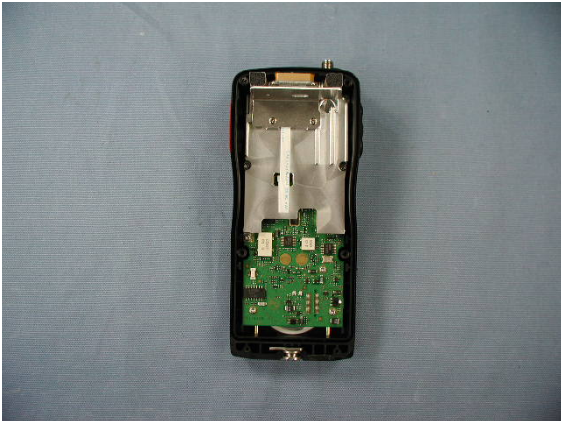
Removed Rear Panel with GPS Module
