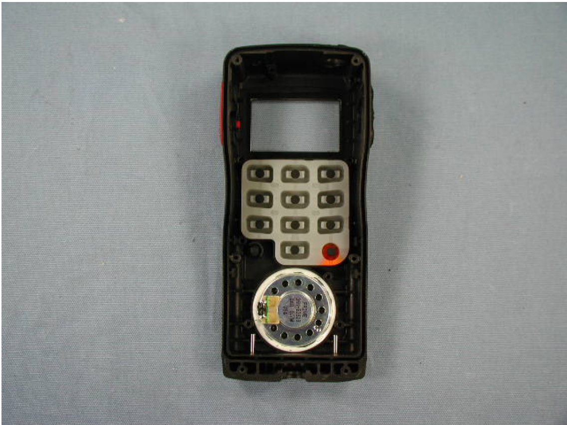
Inside of front panel
