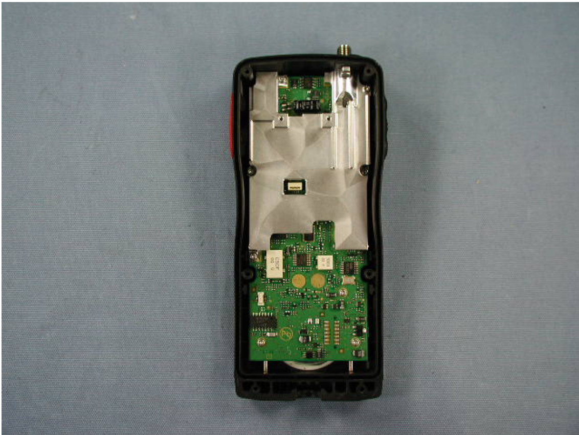
Removed Rear Panel without GPS Module
