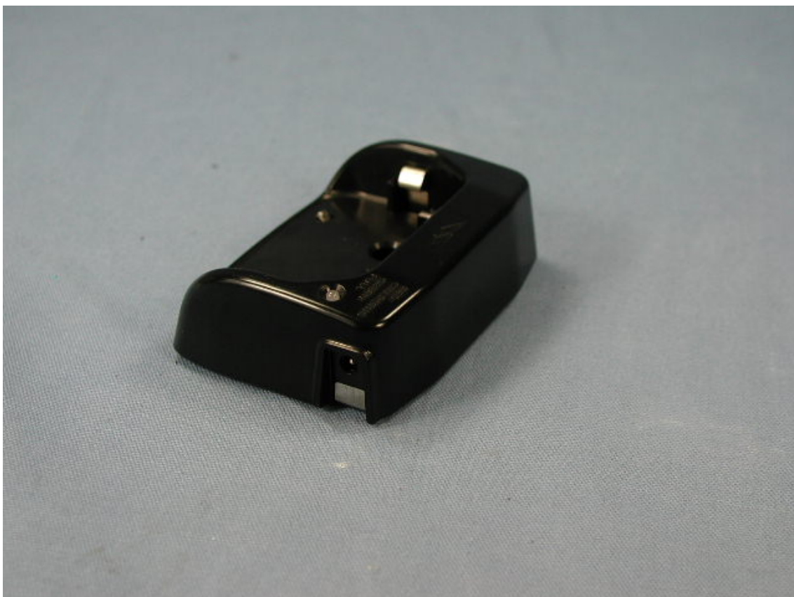
Side of Battery Charger (CD-38)
