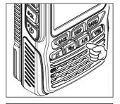
2 Rotate the VOL knob clockwise/counterclockwise to adjust the volume level.
