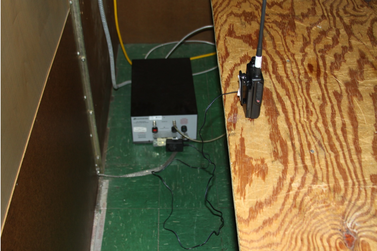
Powerline Conducted Emissions test set up photos
