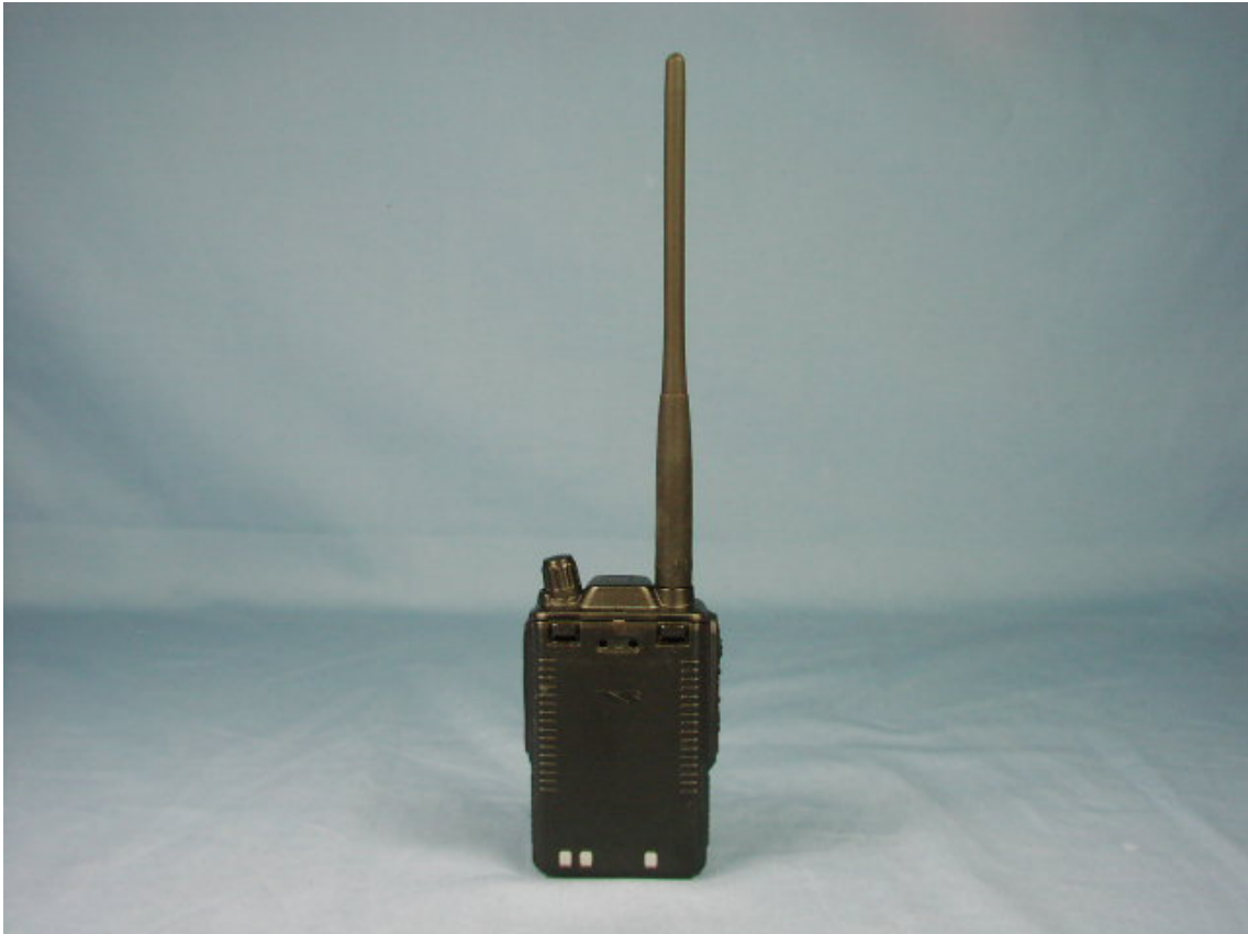
Rear view with Battery Pack and Antenna
