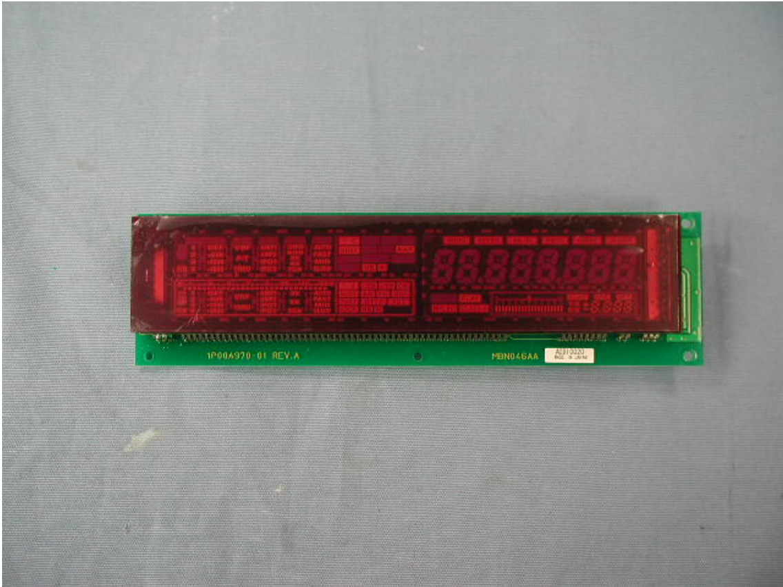
Side-A of VFD-UNIT
