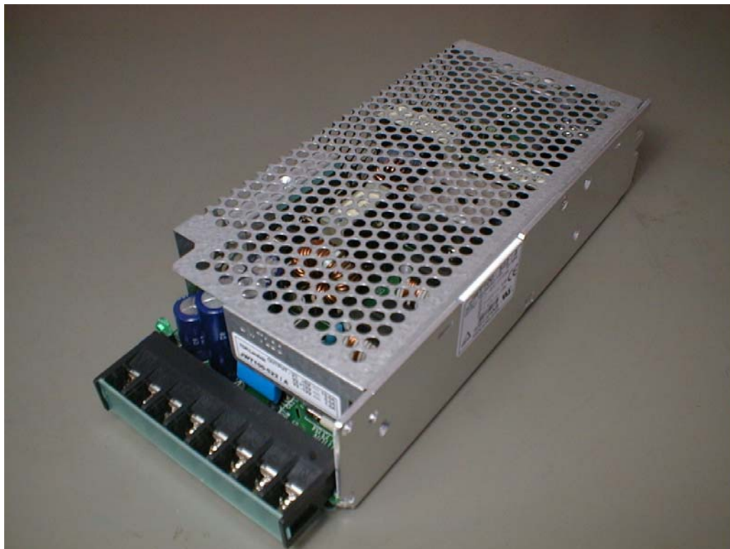
View of POWER SUPPLY UNIT X 1 (+12 / -12 V)
