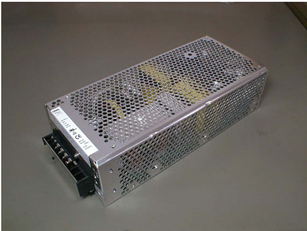
View of POWER SUPPLY UNIT X3 Parallel Connection (48 V)
