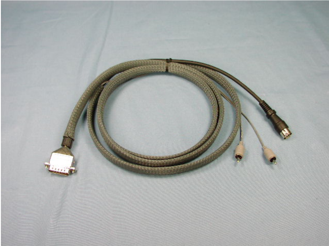
View of Control Cable (BAND DATA, ALC)
