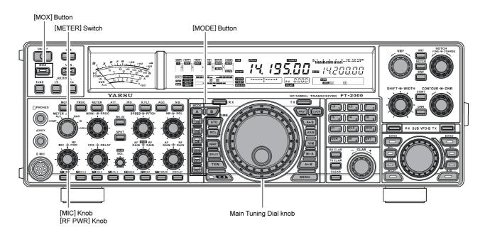
The operating mode is selected using the [MODE] buttons to the left of the Main Tuning Dial knob, and the VFO (A or B) to which the selection is applied is selected by the [A] or [B] button above the [MODE] buttons. Usually, the [A] button glows Red, signifying
