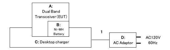
Note: This EUT was tested and certificated with below Configuration B. Then, manufacturer change the charging specification that the EUT cannot charge a battery with this configuration. After this change, the EUT can charge with above Configuration A only. For this reason, the EUT was re-tested with Configuration A in this report.
