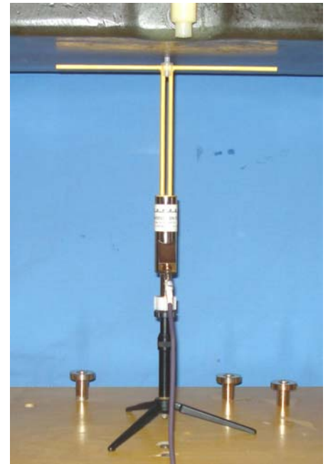
SPEAG 450 MHz Validation Dipole Setup
