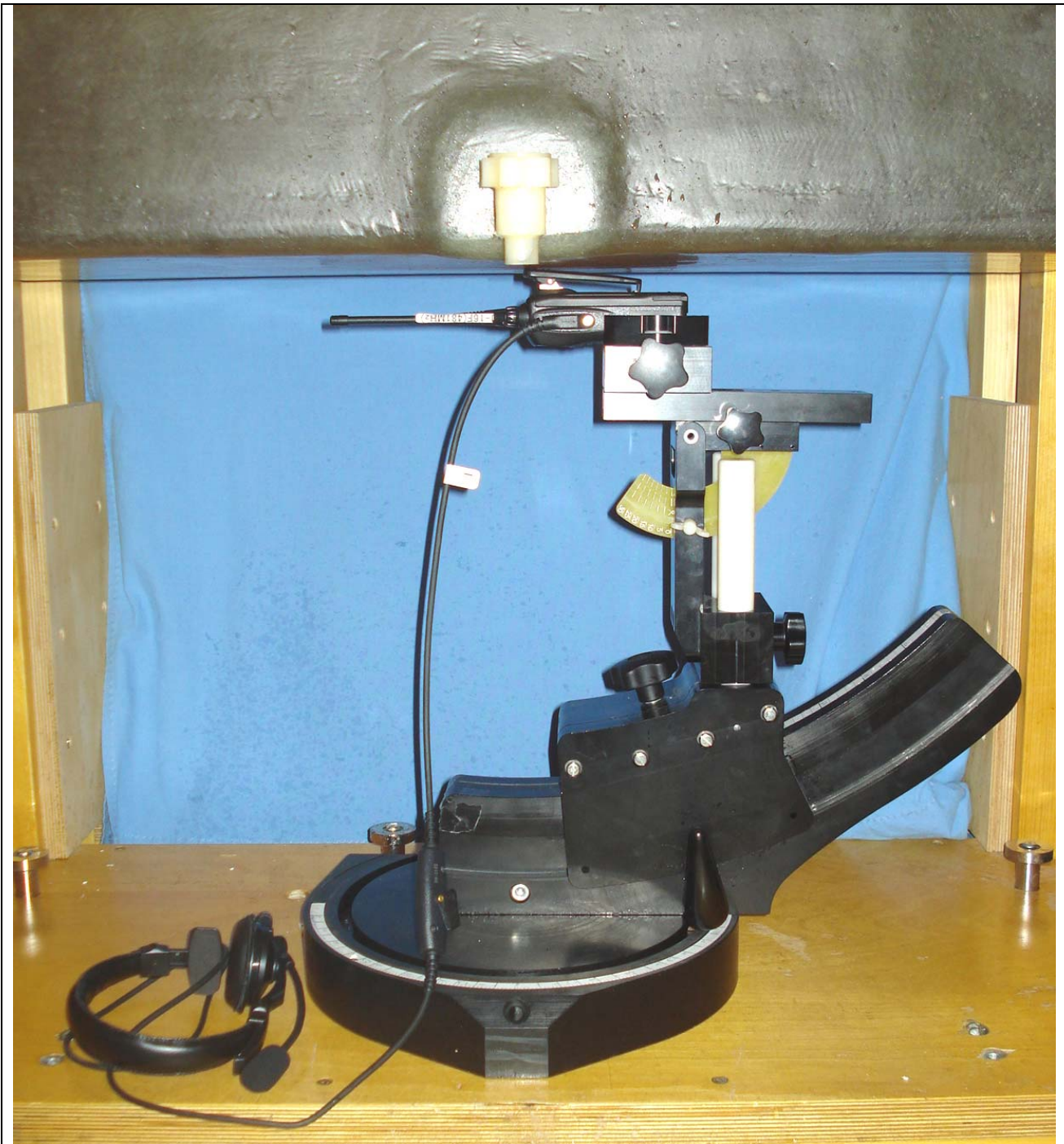
DUT with Belt-Clip Body-worn Accessory (P/N: CLIP-20) & Audio Accessory Category #1 (Headset P/N: VH-215S)
