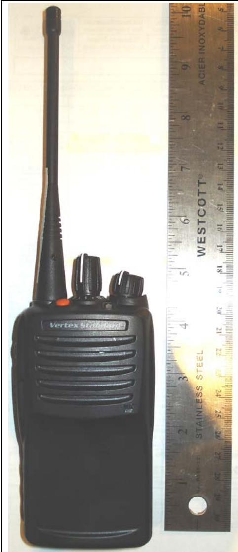
Front of VX-451-G7-5 Radio & Antenna B with ATU-16F Antenna (B)
