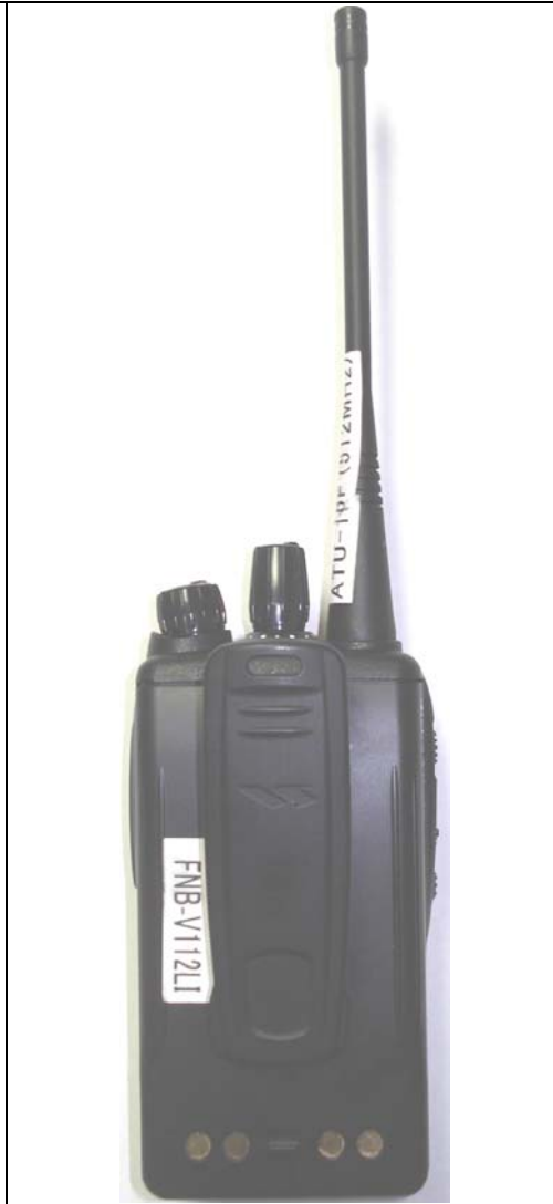
Back of VX-459-G7-5 Radio & Antenna B with Standard Li-ion Battery (a)
