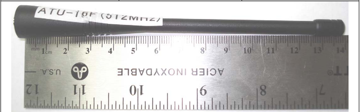
Whip Antenna (B) P/N: ATU-16F (Length = 138 mm)
