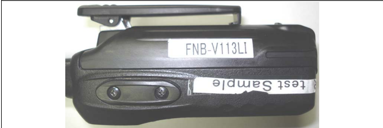
Right Side of Radio with Belt-Clip & Extended Li-ion Battery (b)
