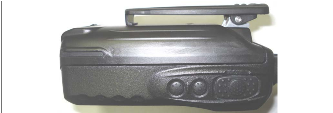
Left Side of Radio with Belt-Clip & Extended Li-ion Battery (b)
