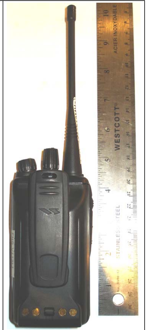
Back of VX-451-G7-5 Radio & Antenna B with Extended Li-ion Battery (b)
