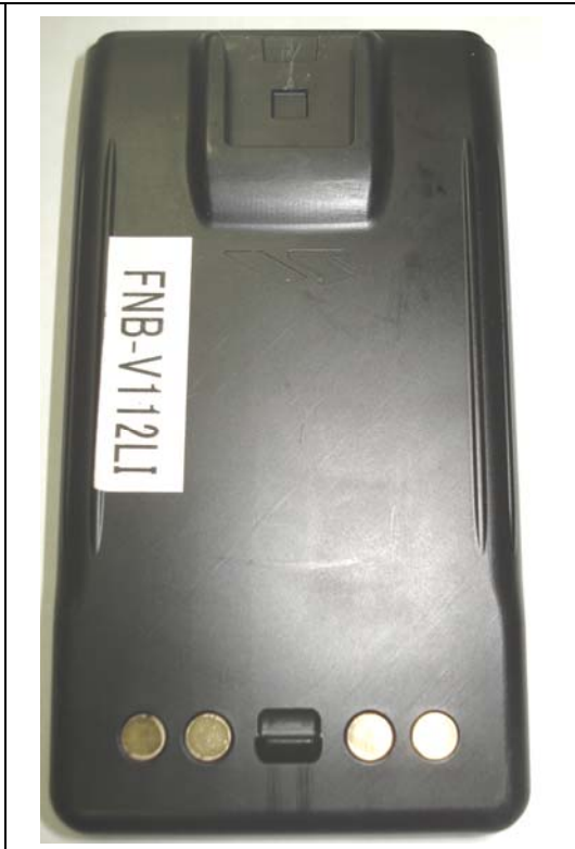
Standard Li-Ion Battery (a) without Belt-Clip
