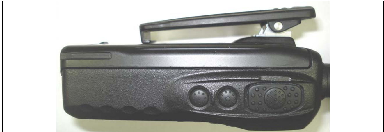
Left Side of Radio with Belt-Clip & Standard Li-ion Battery (a)
