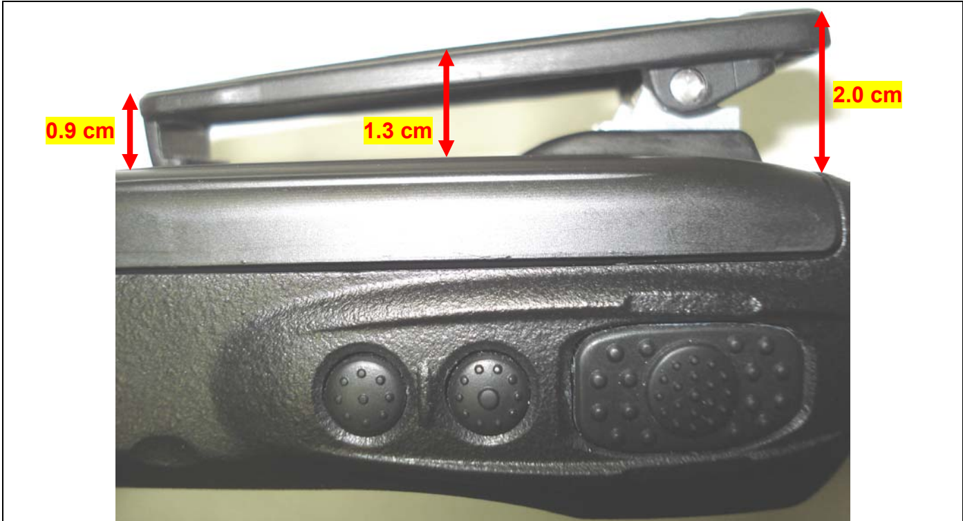
Belt-Clip Thickness Measurement Distance – Radio with Standard Li-ion Battery (a)
