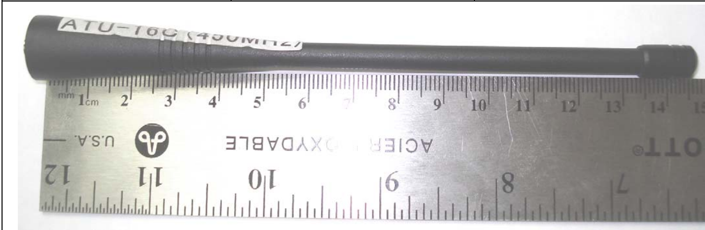
Whip Antenna (A) P/N: ATU-16D (Length = 145 mm)
