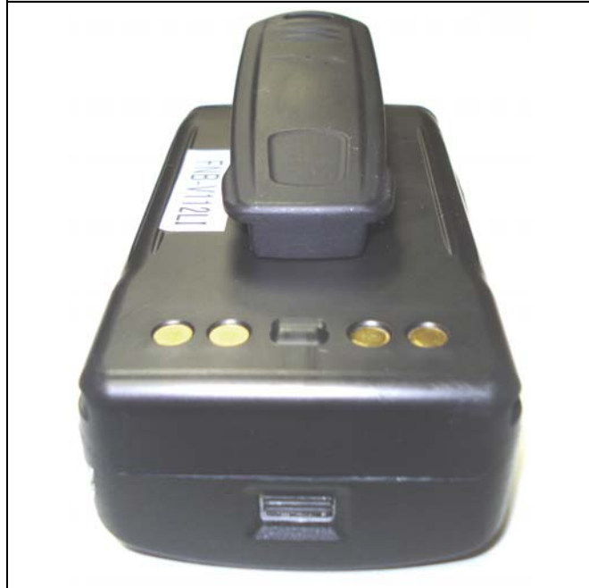
Bottom end of Radio w/ Belt-Clip & Standard Li-ion Battery (a)
