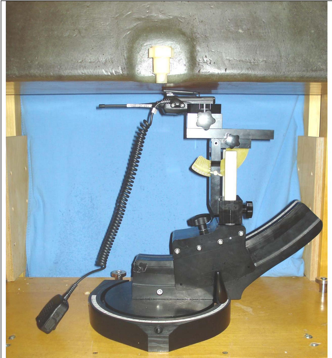
DUT with Belt-Clip Body-worn Accessory (P/N: CLIP-20) & Audio Accessory Category #3 (Speaker-Mic P/N: MH-45B4B)
