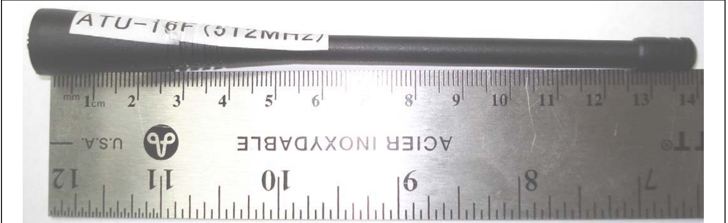
Whip Antenna (B) P/N: ATU-16F (Length = 138 mm)
