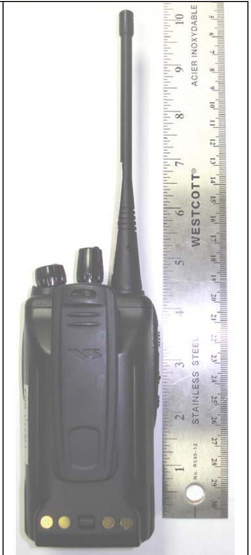
Back of Radio w/ Extended Li-ion Battery (b)
