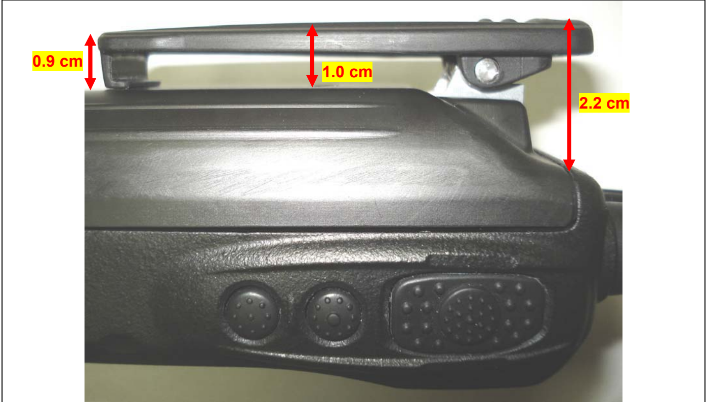
Belt-Clip Thickness Measurement Distance – Radio with Extended Li-ion Battery (b)
