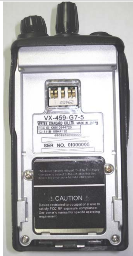
Back of Radio with Battery removed
