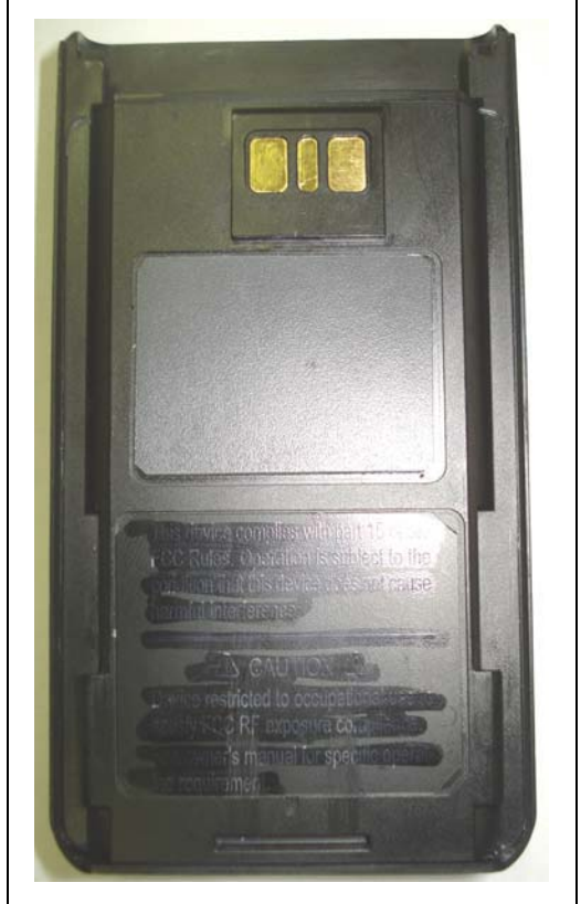
Extended Li-Ion Battery (b) - 2400 mAh
