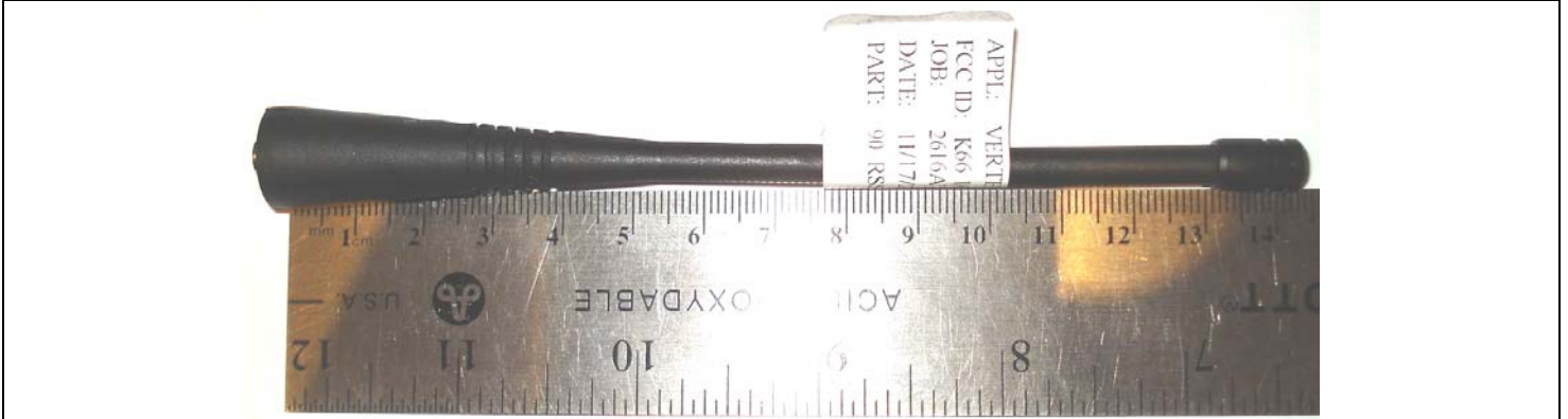
Whip Antenna (C) P/N: ATU-16D (Length = 143 mm)
