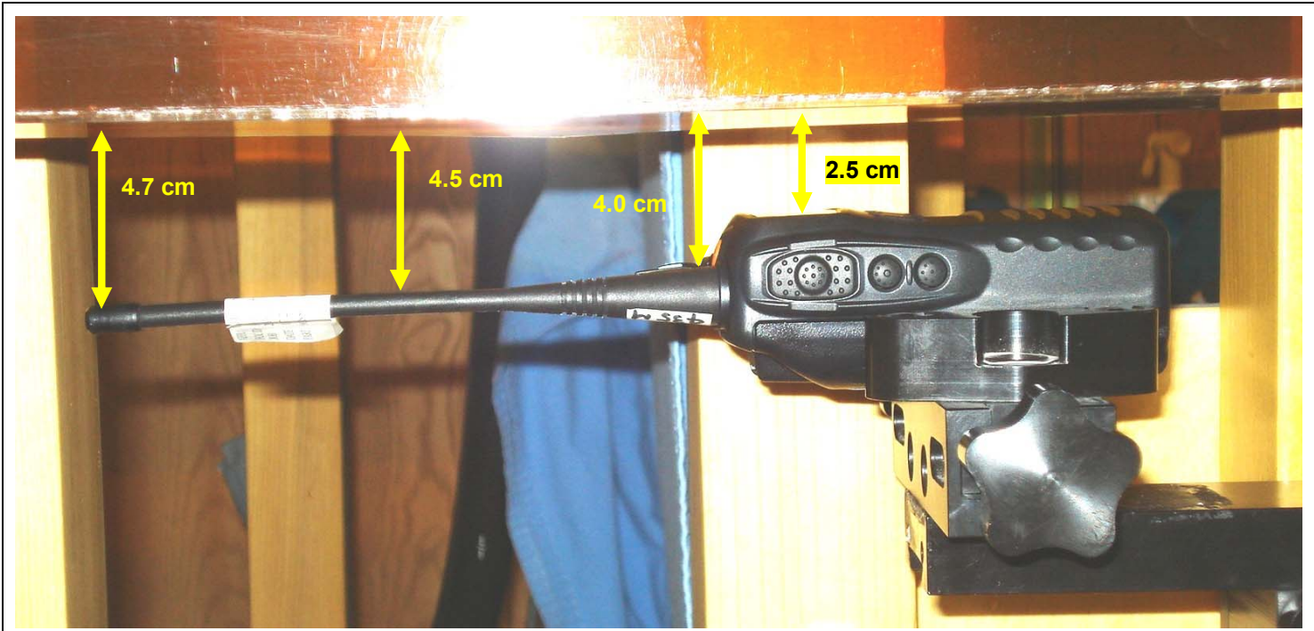
Face-held - VX-454-G6-5 Radio with ATU-16C Antenna (B) & Li-Ion Extended Battery (b)
