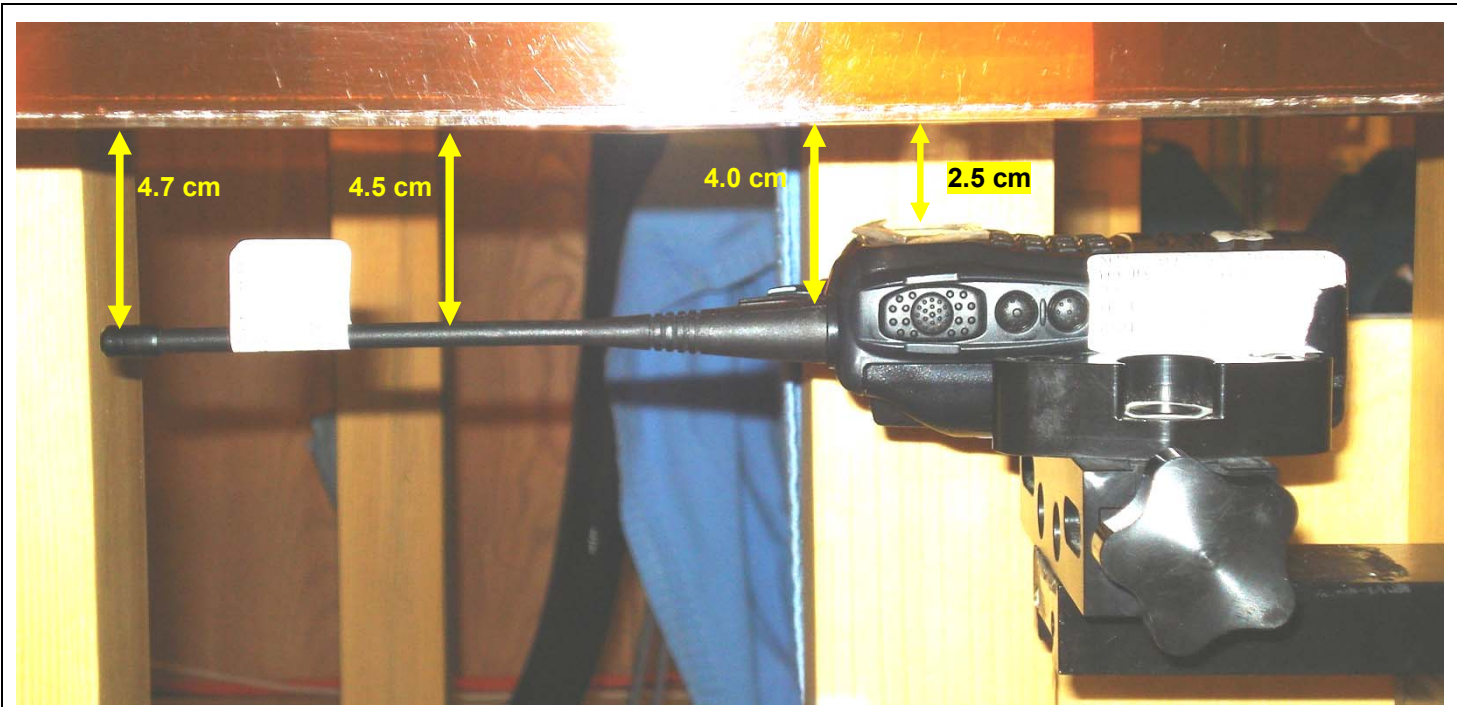
Face-held - VX-459-G6-5 Radio with ATU-16B Antenna (A) & Li-Ion Extended Battery (b)
