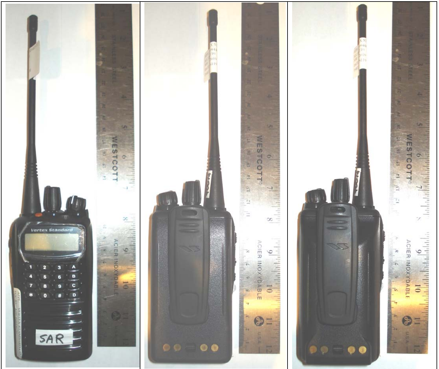
Front of VX-459-G6-5 Radio with ATU-16B Antenna (A) Back of VX-459-G6-5 Radio & Antenna A with Standard Li-ion Battery (a) Back of VX-459-G6-5 Radio & Antenna A with Extended Li-ion Battery (b)
