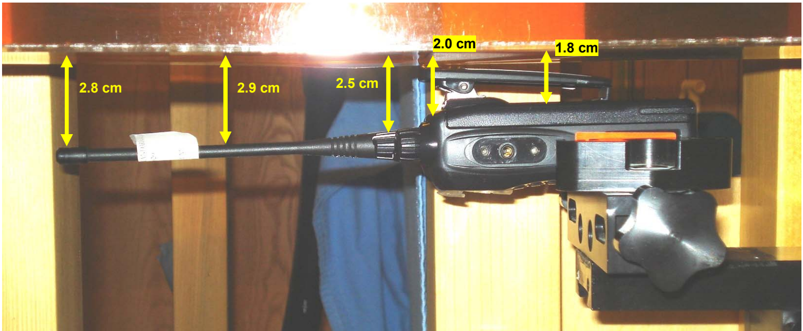
Body-worn – VX-459-G6-5 Radio with ATU-16C Antenna (B) & Li-Ion Standard Battery (a) - 1.8 cm Belt-Clip Spacing (Battery Housing & Antenna Parallel to Phantom)
