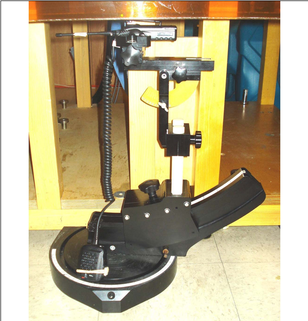
DUT with Belt-Clip Body-worn Accessory (P/N: CLIP-20) & Audio Accessory Category #3 (Speaker-Mic P/N: MH-45B4B)
