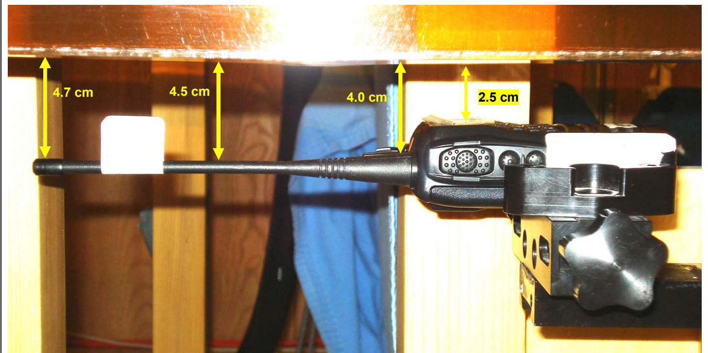
Face-held - VX-459-G6-5 Radio with ATU-16B Antenna (A) & Li-Ion Standard Battery (a)
