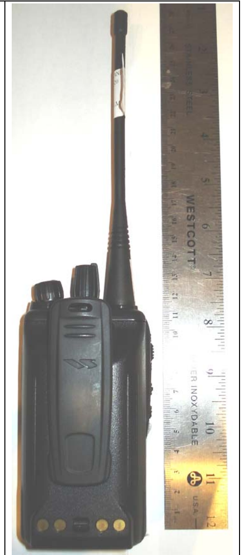
Back of VX-459-G6-5 Radio & Antenna B with Extended Li-ion Battery (b)
