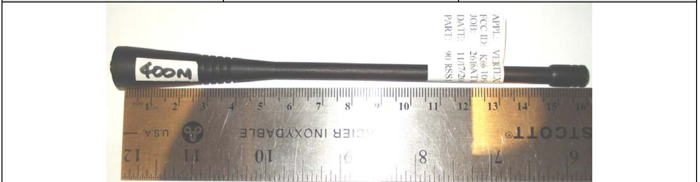
Whip Antenna (A) P/N: ATU-16B (Length = 160 mm)
