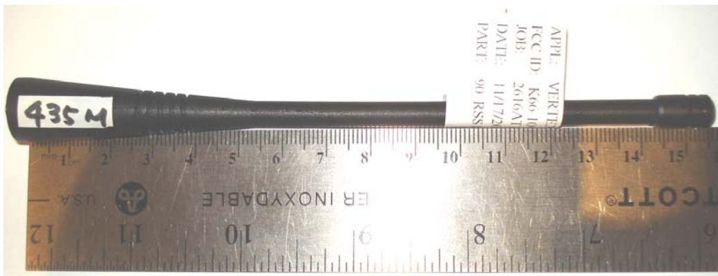
Whip Antenna (B) P/N: ATU-16C (Length = 155 mm)
