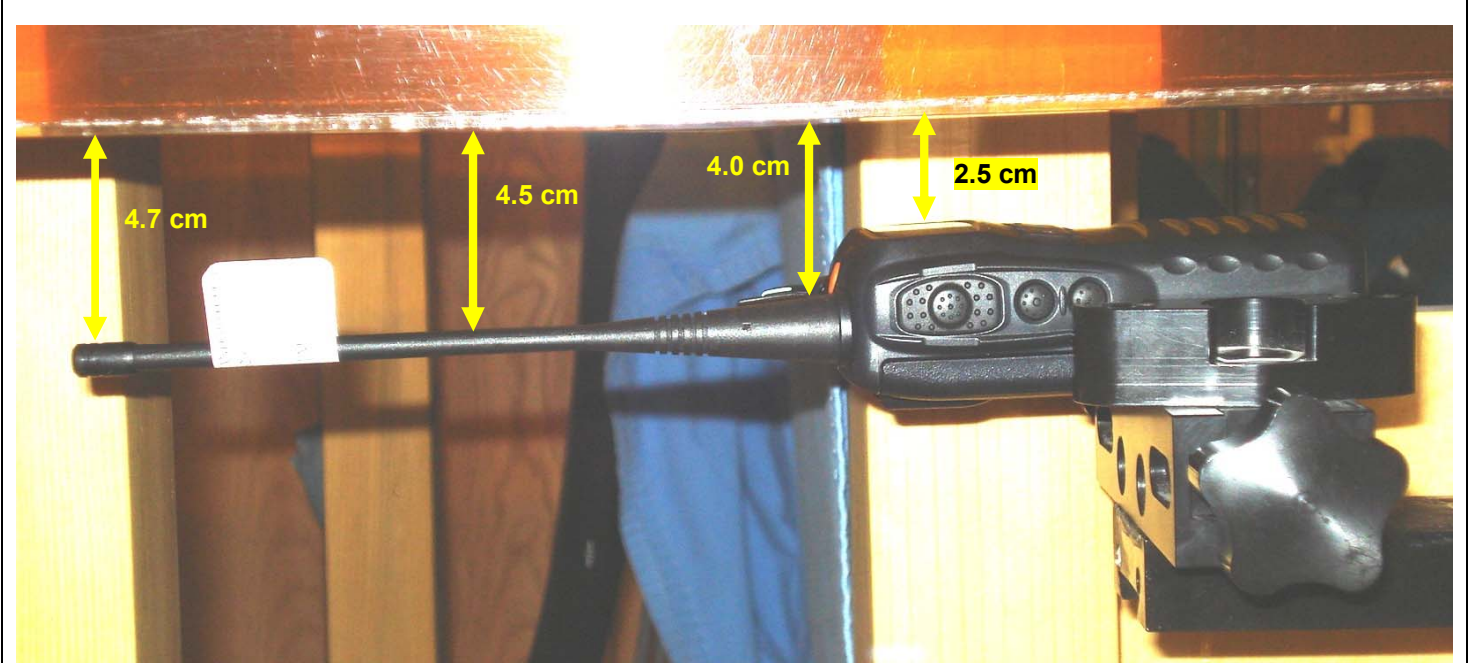
Face-held - VX-454-G6-5 Radio with ATU-16B Antenna (A) & Li-Ion Standard Battery (a)
