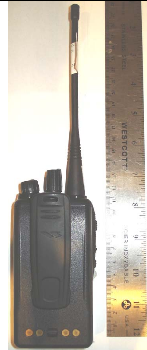
Back of VX-459-G6-5 Radio & Antenna B with Standard Li-ion Battery (a)
