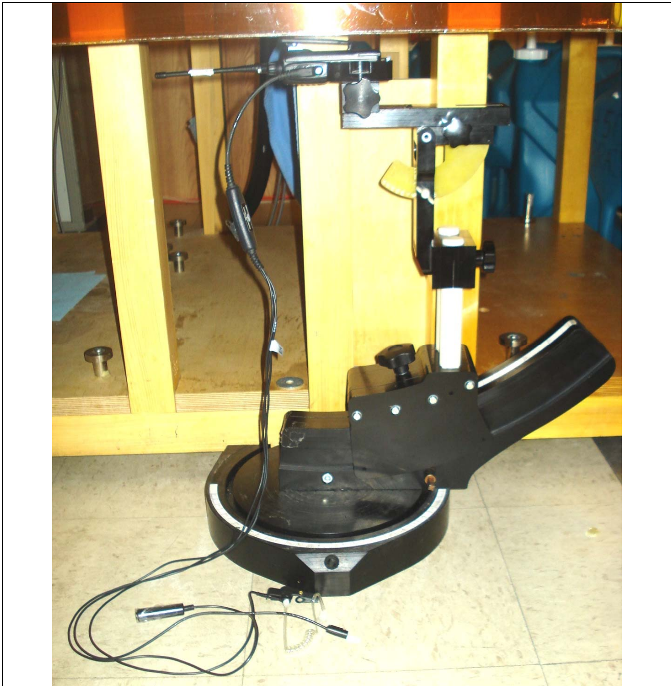
DUT with Belt-Clip Body-worn Accessory (P/N: CLIP-20) & Audio Accessory Category #2 (Earpiece w/ mic/PTT P/N: VH-120S)
