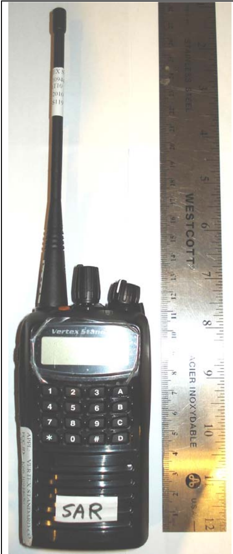
Front of VX-459-G6-5 Radio with ATU-16C Antenna (B)
