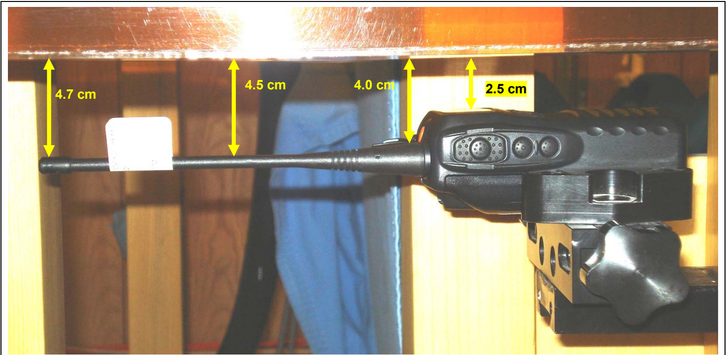
Face-held - VX-454-G6-5 Radio with ATU-16B Antenna (A) & Li-Ion Extended Battery (b)
