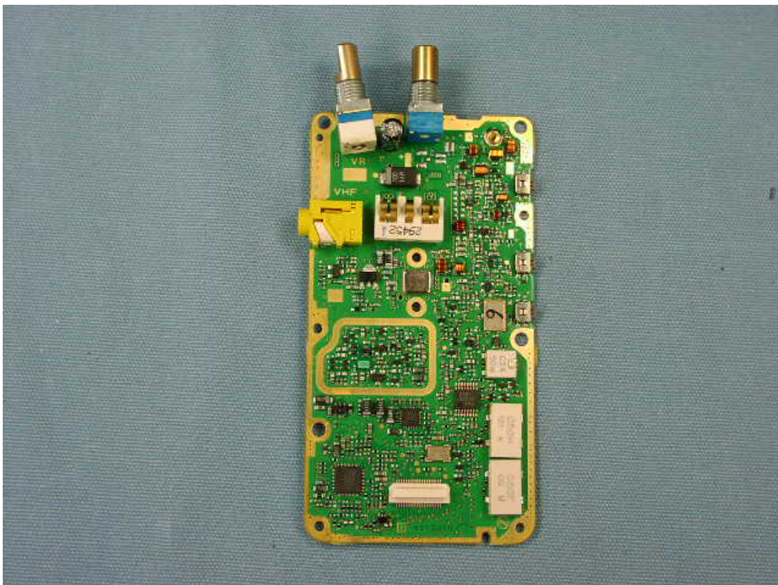
Side A of MAIN-UNIT Without VCO Case (VX-451 / VX-454 / VX-459)
