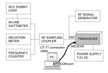
The transceiver must be programmed for use in the intended system before alignment is attempted. The RF parameters are loaded from the file during the alignment process.
