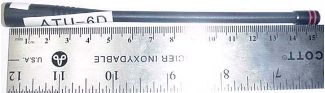
Whip Antenna P/N: ATU-6D (450-485 MHz)
