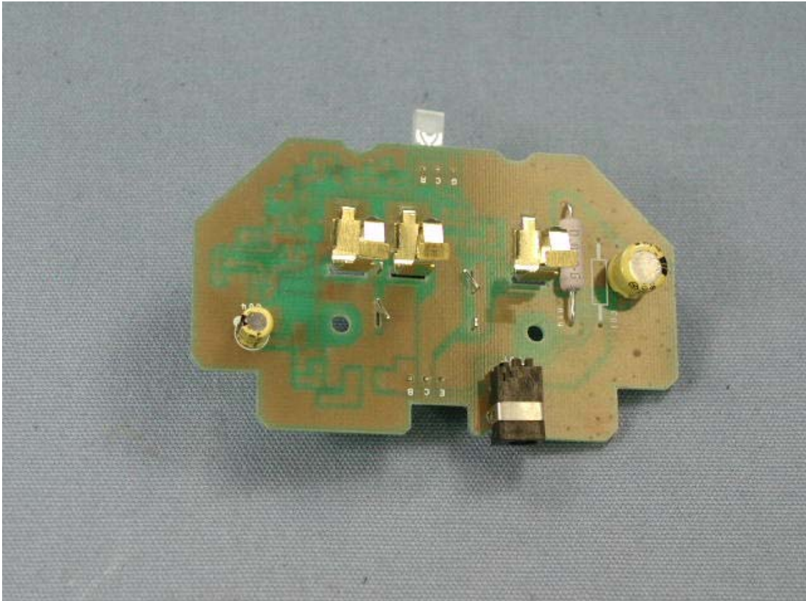
PWB of Battery Charger
