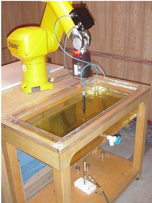
DASY4 SAR System with Plexiglas validation phantom
