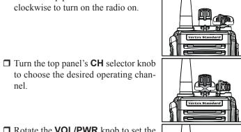
☐ Rotate the **VOL/PWR** knob to set the volume level. If no signal is present, press and hold in the **Programmable** key assigned to "SQL OFF" for more than one second; background noise will now be heard, and you may use this to
