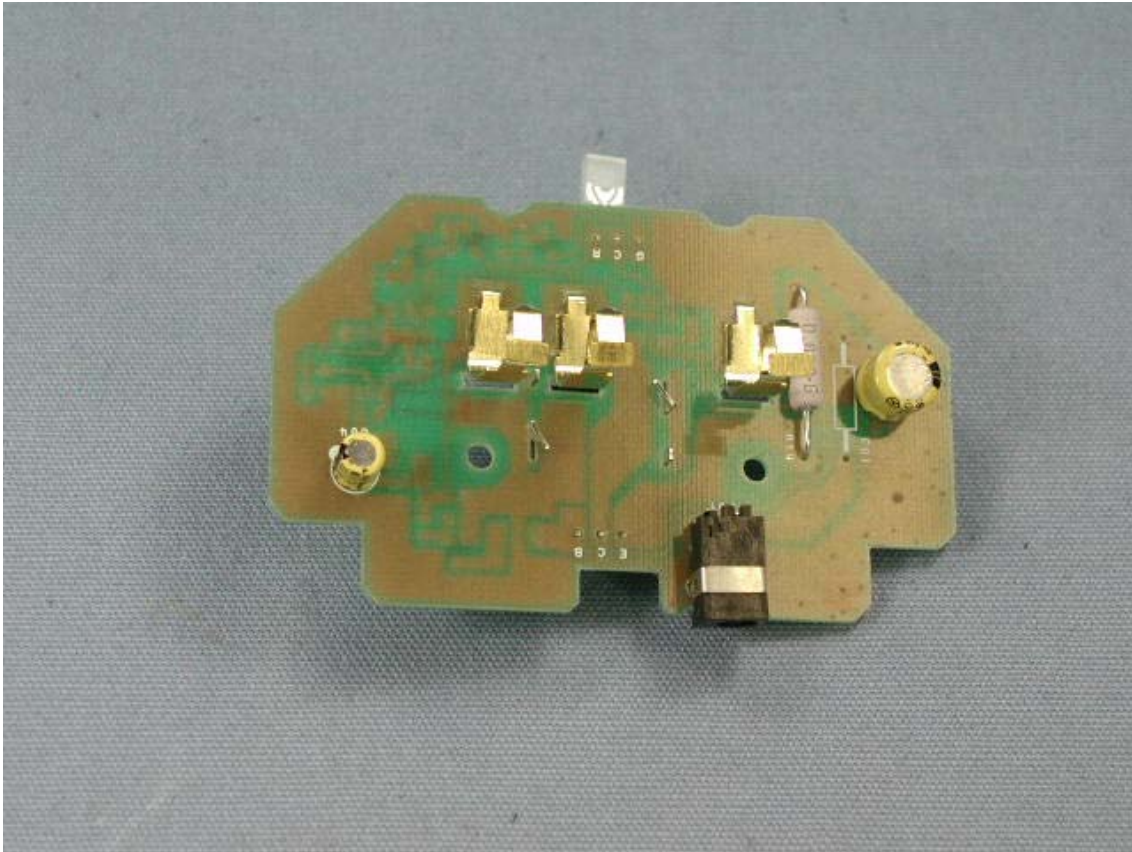
PWB of Battery Charger
