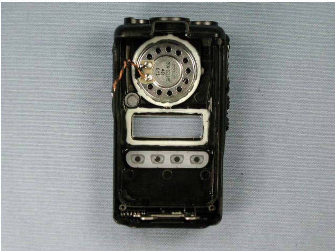
Inside of front panel (for VX-354)
