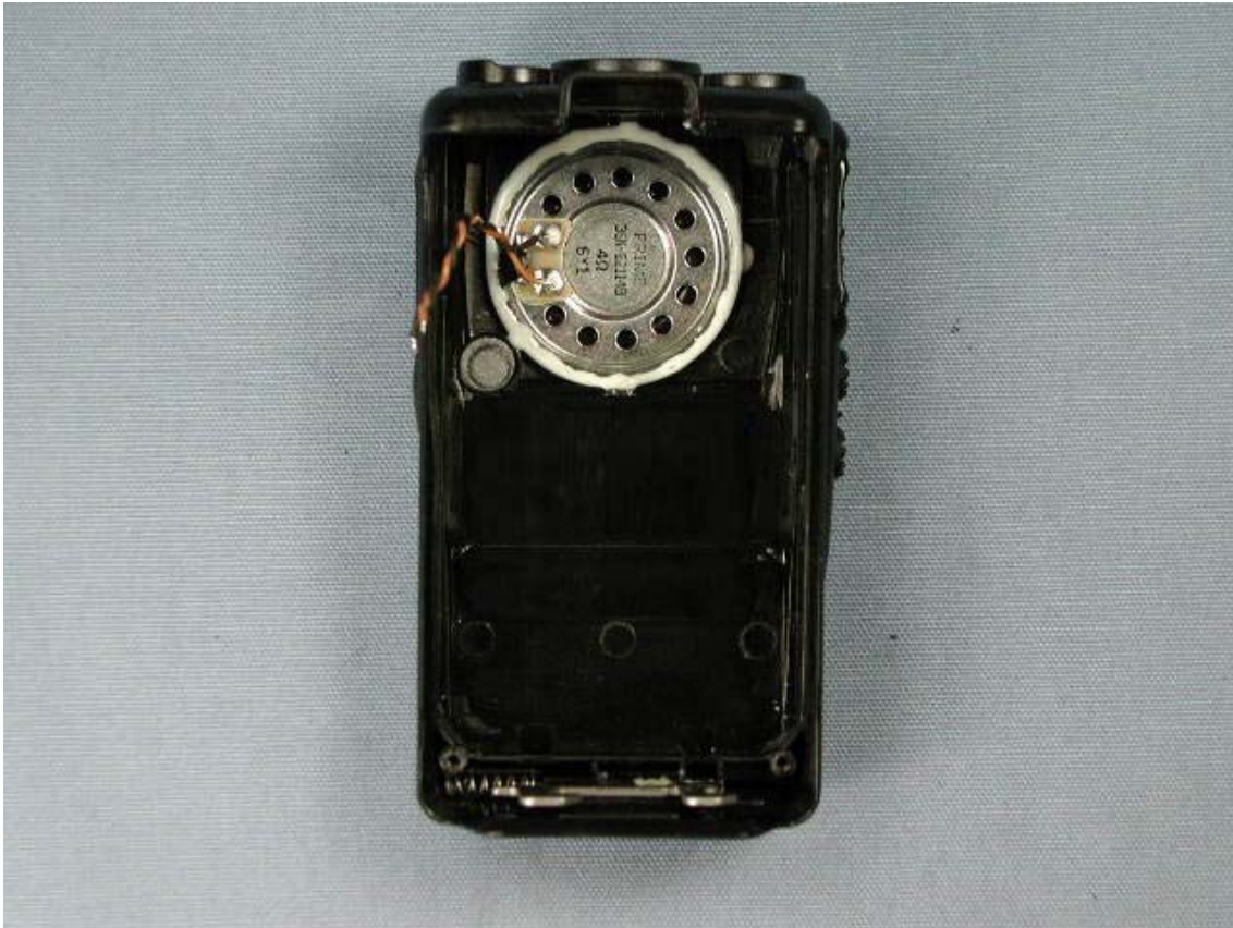
Inside of front panel (for VX-351)
