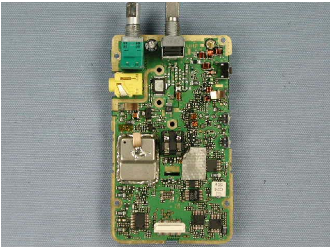
Side-B of MAIN-3-UNIT with shield cases
