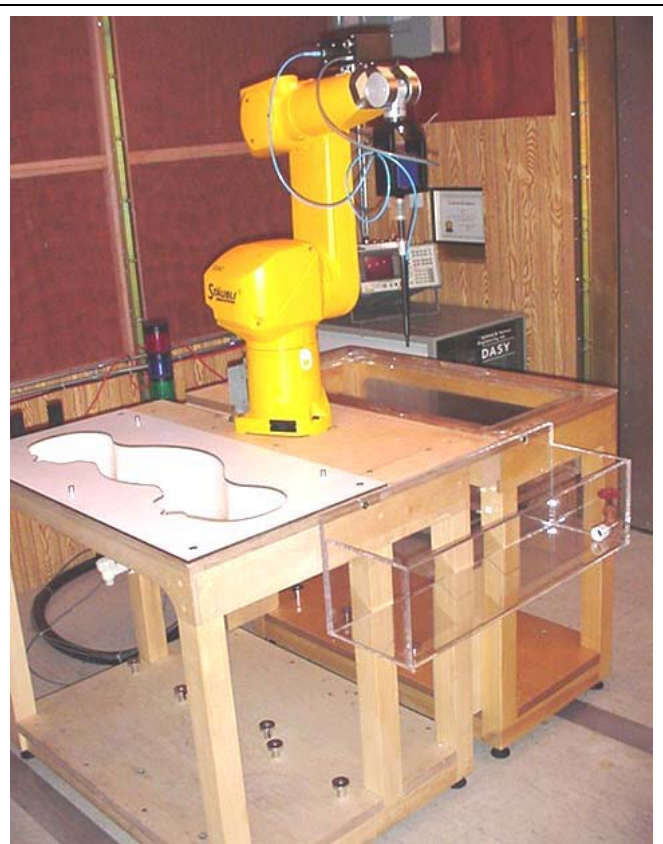
DASY4 SAR Measurement System with Plexiglas side planar phantom
