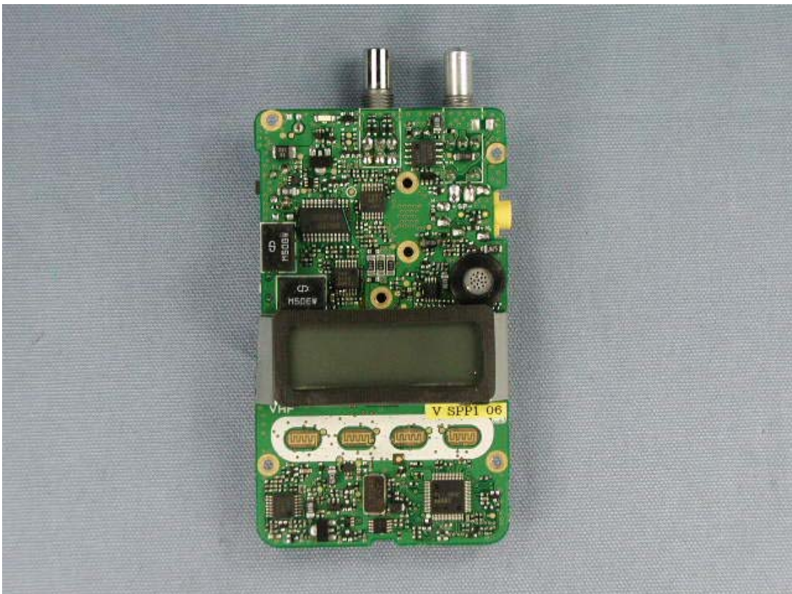
Side-A of MAIN-UNIT with LCD
