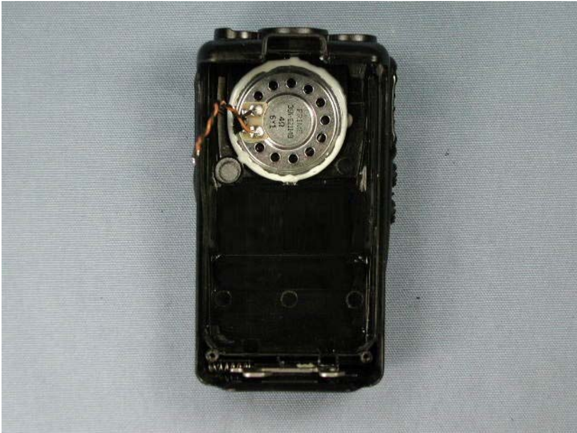
Inside of front panel (for VX-351)
