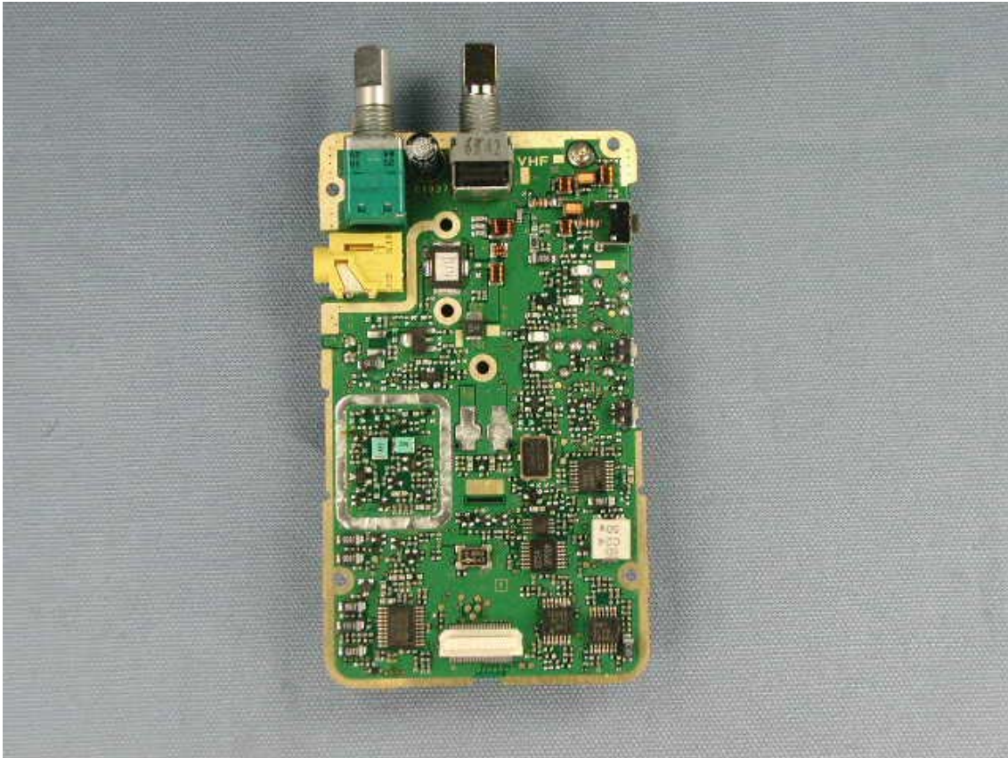
Side-B of MAIN-UNIT without shield cases
