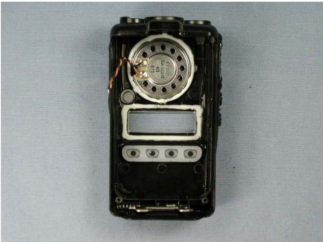
Inside of front panel (for VX-354)
