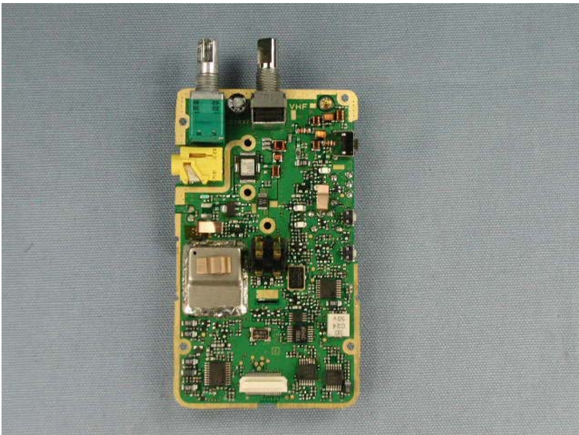
Side-B of MAIN-UNIT with shield cases
