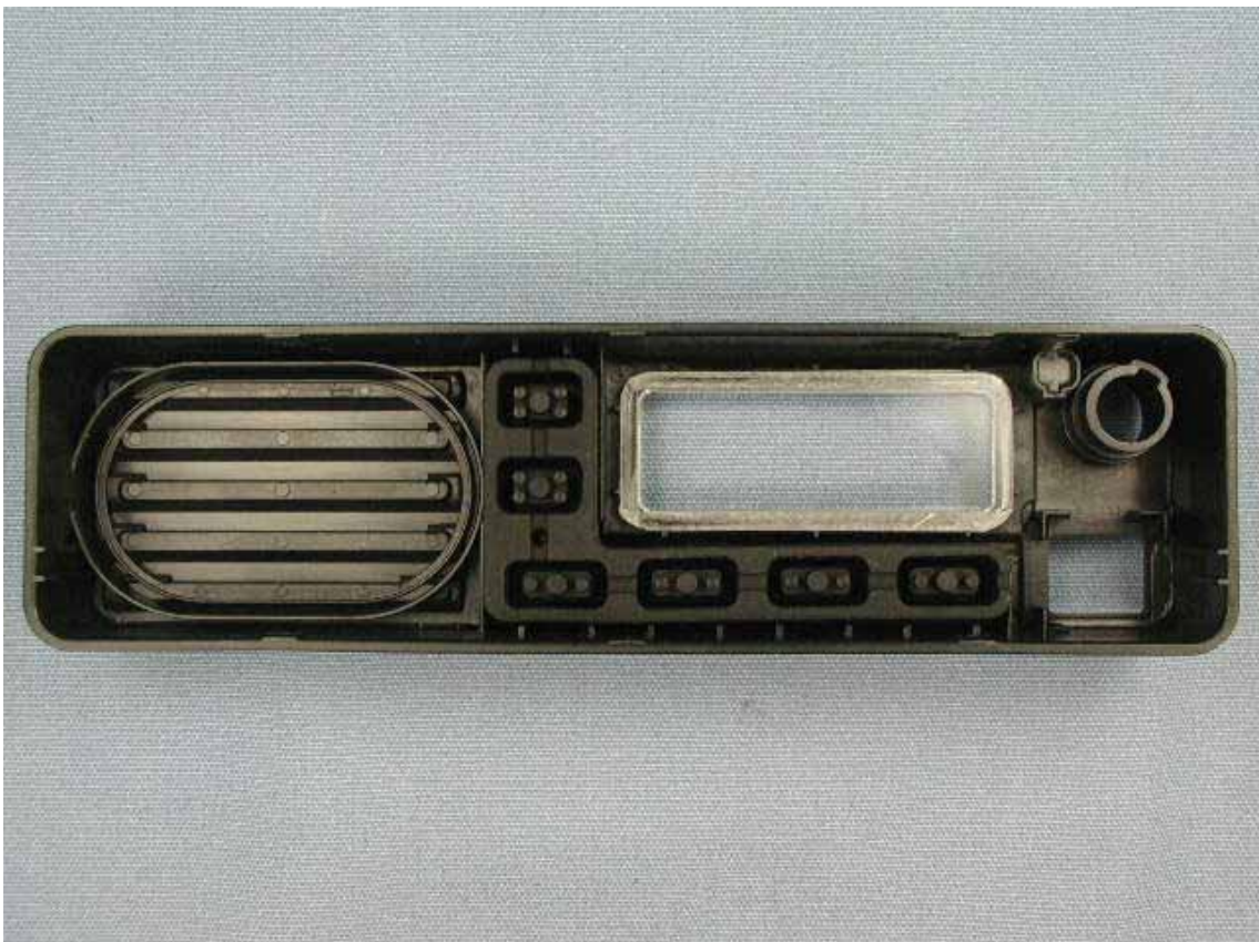
Inside of front panel (VX-2200)
