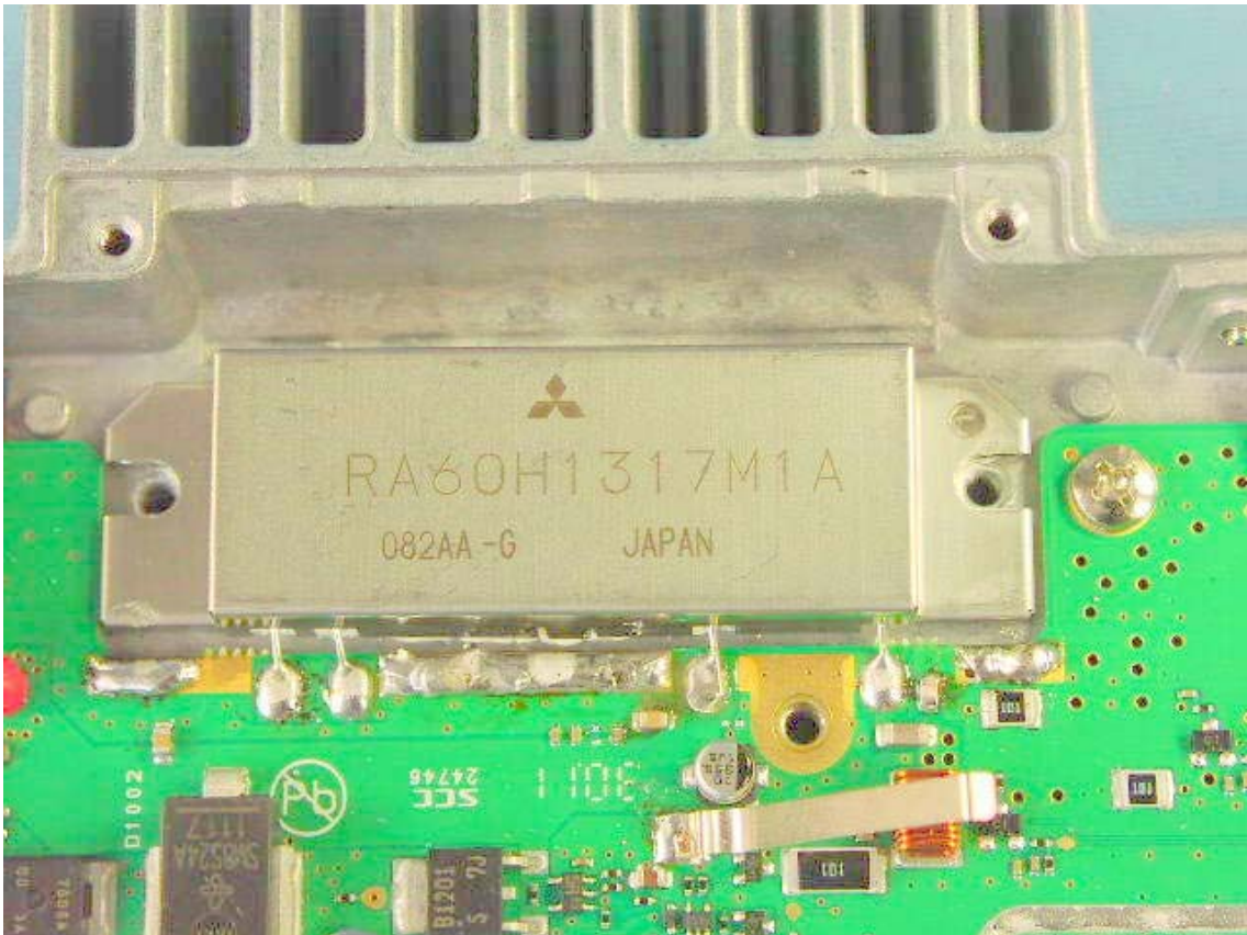
Replacement Power Module without Shield case (Close-up)
