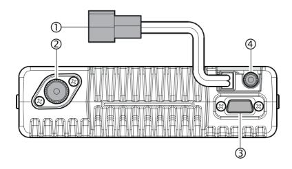
The supplied DC power cable must be connected to this 2-pin connector. Use only the supplied fused cable, extended if necessary, for power connection.
