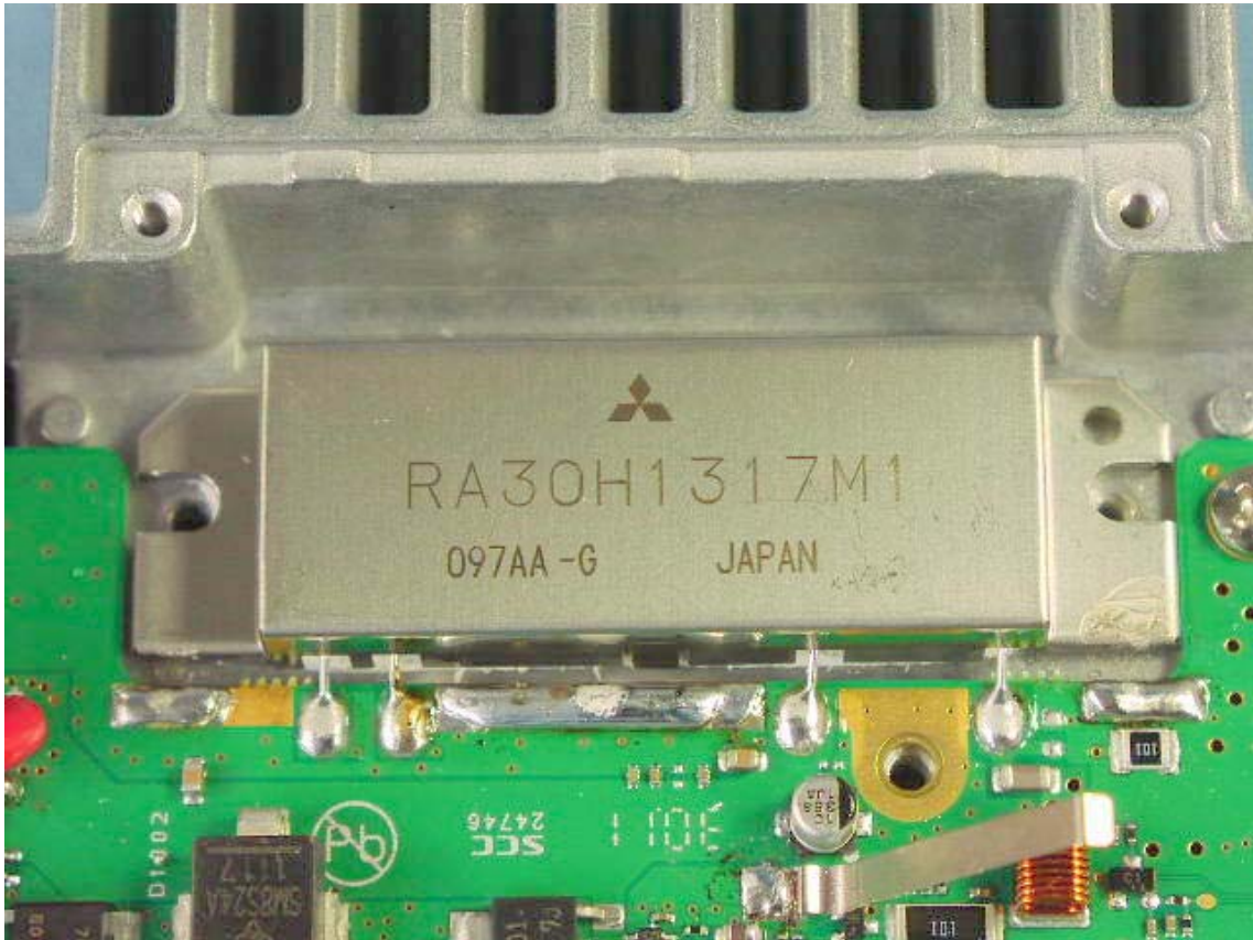
Replacement Power Module (Close-up)
