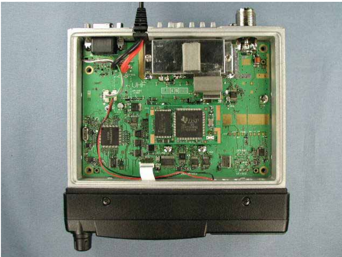
Inside of EUT with shield case and MODEM-UNIT
