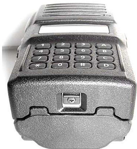
Bottom end of DUT with 2000 mAh Li-ion Battery
