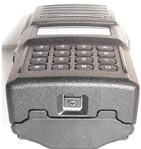
Bottom end of DUT with 1150 mAh Li-ion Battery
