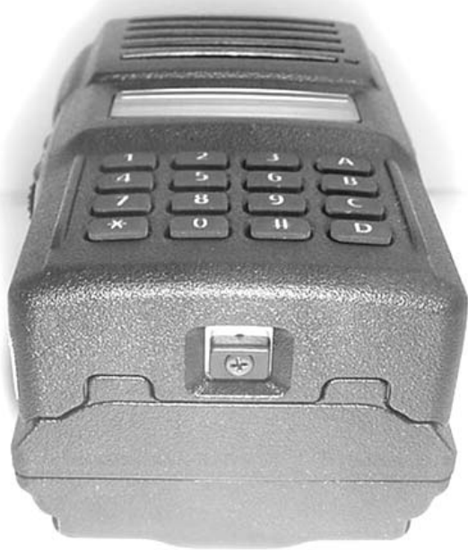
Bottom end of DUT with 3000 mAh Li-ion Battery
