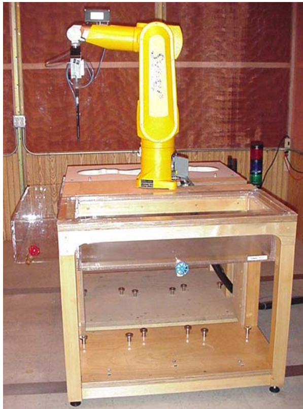
DASY4 SAR Measurement System with validation phantom
