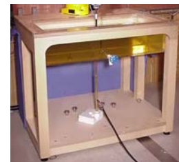
Validation Planar Phantom
