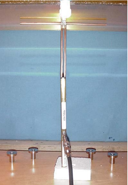
450MHz Dipole Setup
