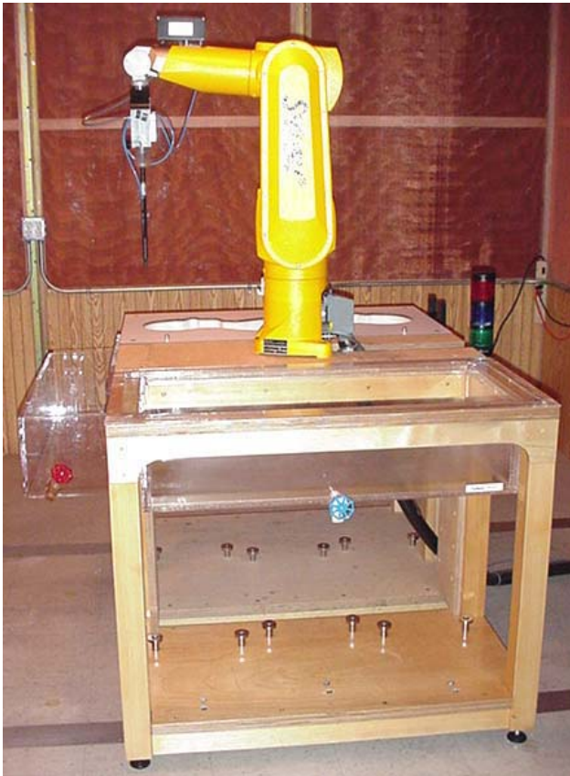
DASY4 SAR Measurement System with validation phantom
