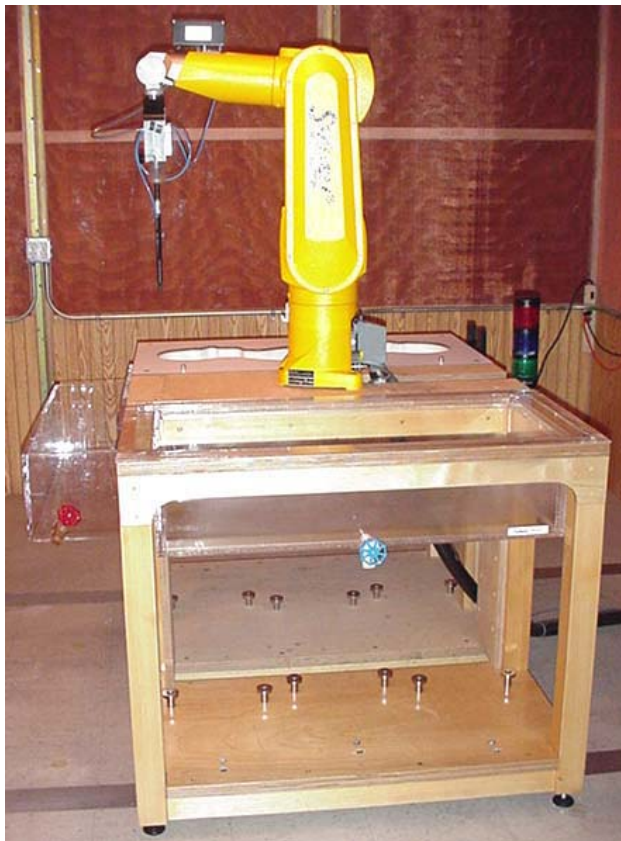
DASY4 SAR Measurement System with validation phantom
