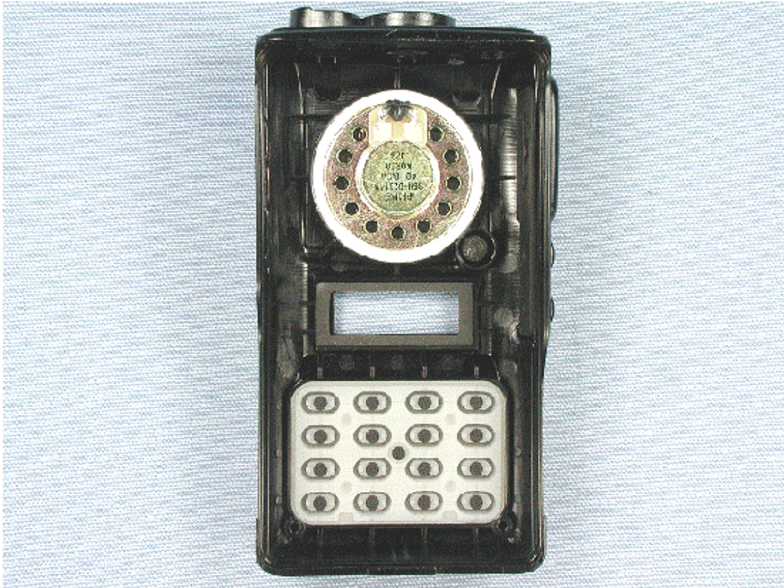
Inside of front panel (VX-424)
