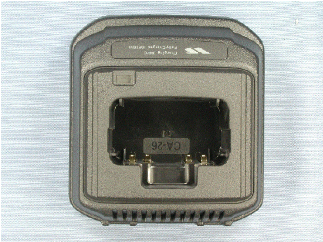
Top of Battery Charger
