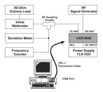
The **VXR-9000** must be programmed for use in the intended system before alignment is attempted. The RF parameters are loaded from the file during the alignment process.
