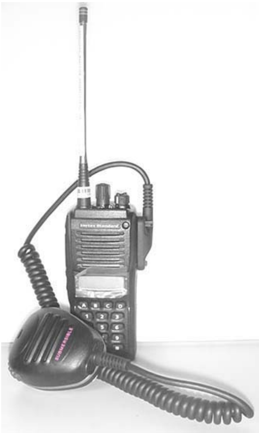
DUT with Speaker-Microphone Audio Accessory (P/N: MH-65B7A)
