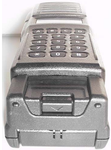
Bottom of DUT with Alkaline Battery Case
