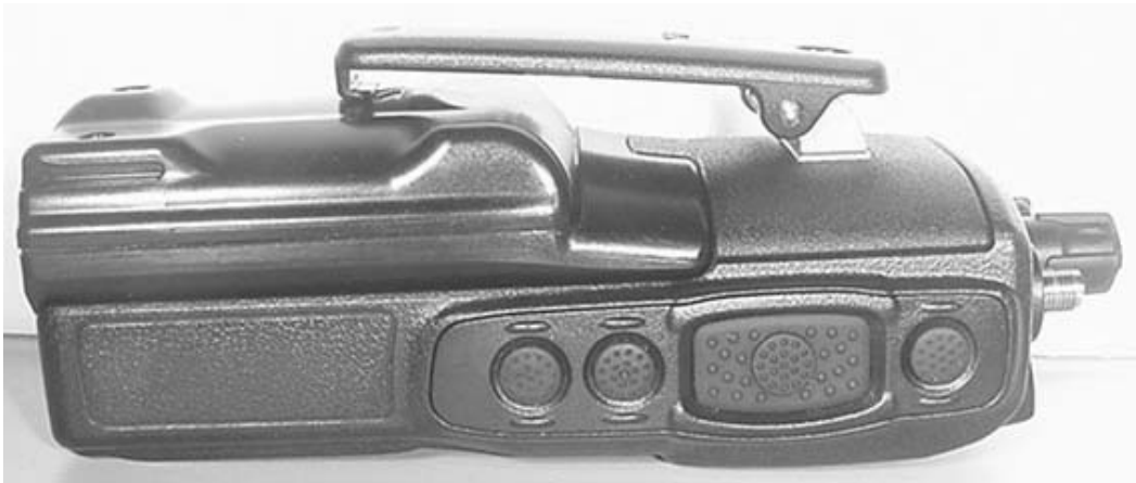
Left Side of DUT with 3000 mAh Li-ion IS Battery & Belt-Clip
