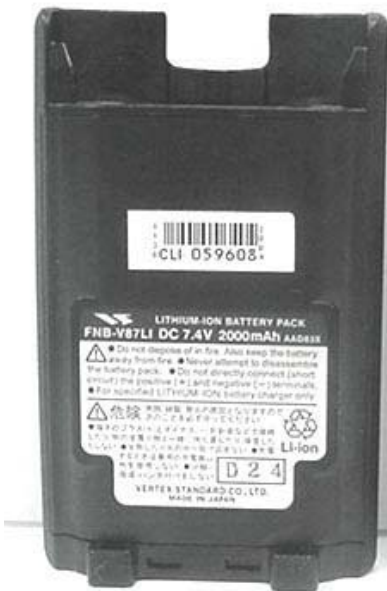
Li-ion Battery 2000 mAh (P/N: FNB-V87LI)
