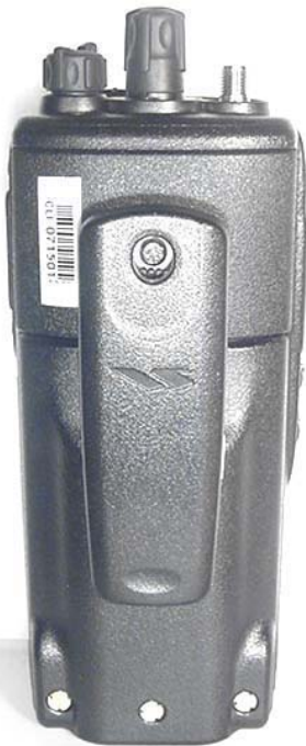
Back of DUT with 2000 mAh Li-ion Battery & Belt-Clip
