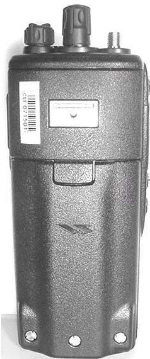
Back of DUT with 1150 mAh Li-ion Battery
