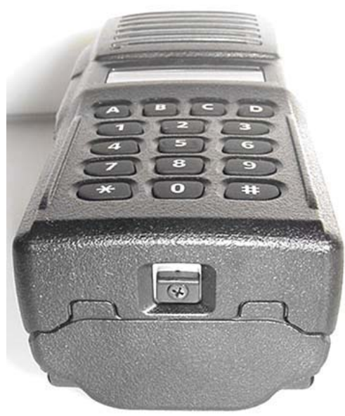
Bottom of DUT with 2000 mAh Li-ion Battery
