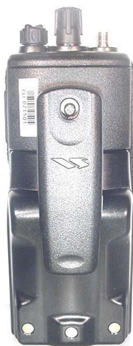
Back of DUT with 3000 mAh Li-ion IS Battery & Belt-Clip
