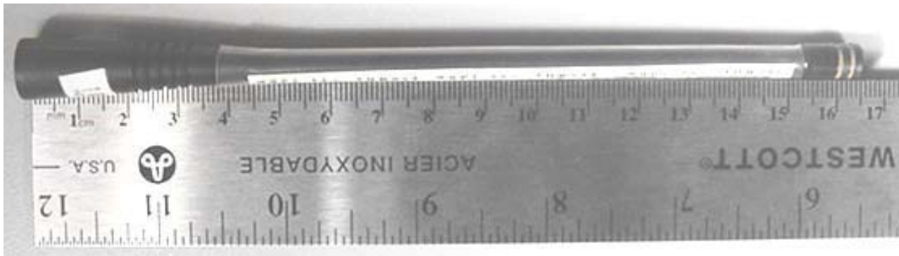
Whip Antenna (P/N: ATU-6A1)
