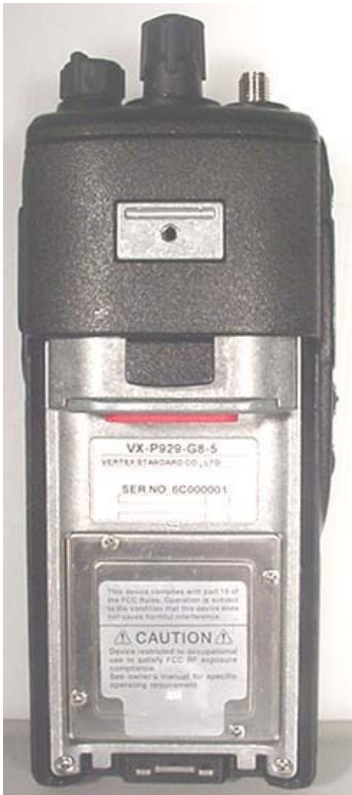
DUT Battery Compartment
