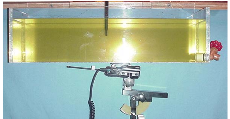
Body-Worn SAR Test Setup Configuration
