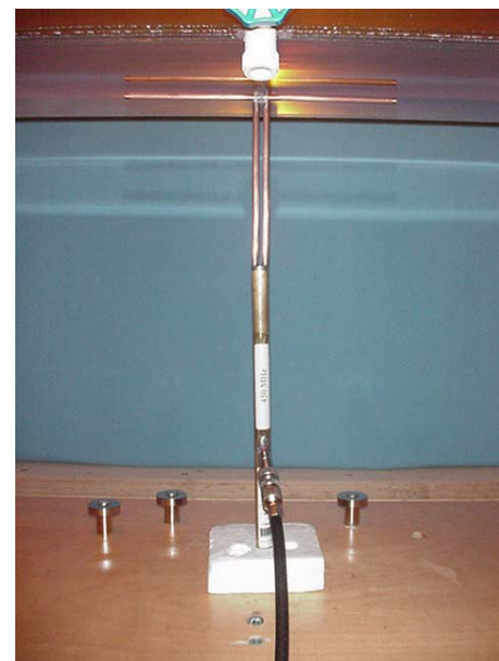
450 MHz Dipole Setup
