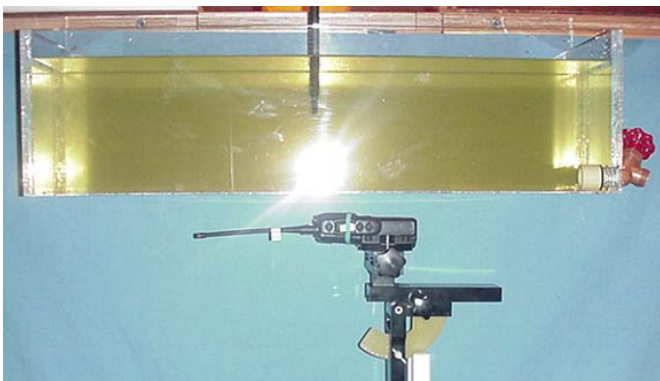
Face-Held SAR Test Setup Configuration
