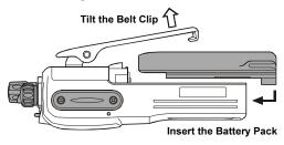
☐ To remove the battery, turn the radio off and remove any protective cases. Slide the Battery Pack Latch on the bottom of the radio toward the front panel while sliding the battery down about 1/2 inch. Then lift the battery out from the radio while unfolding the Belt Clip.
