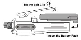
☐ To remove the battery, turn the radio off and remove any protective cases. Slide the Battery Pack Latch on the bottom of the radio toward the front panel while sliding the battery down about 1/2 inch. Then lift the battery out from the radio while unfolding the Belt Clip.
