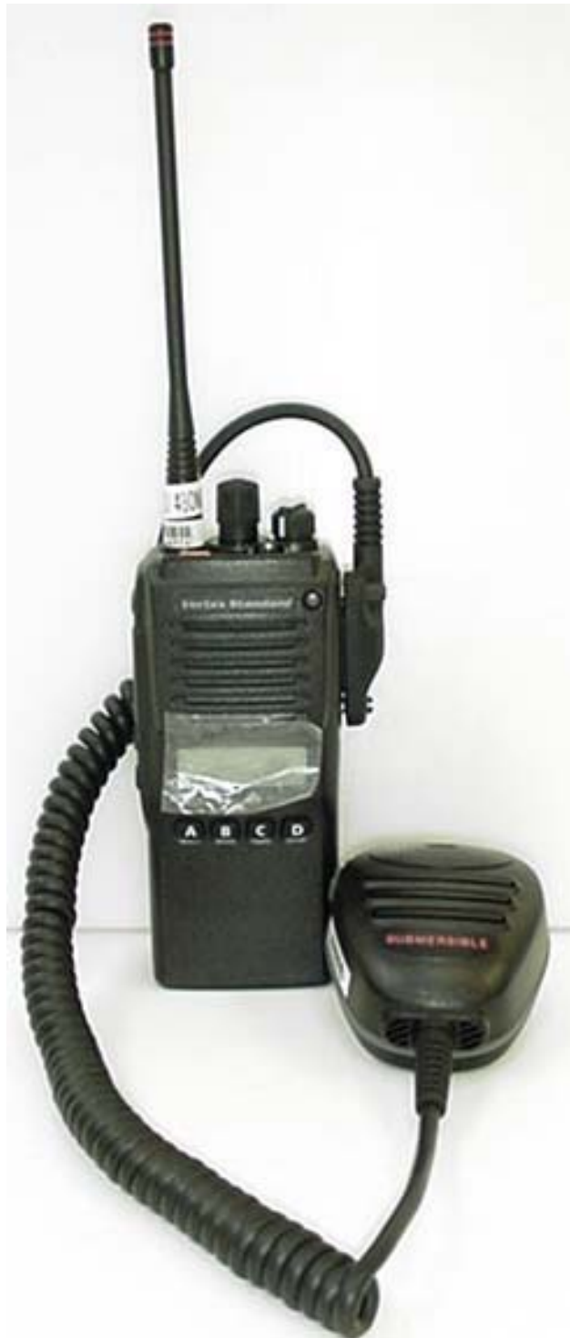
DUT with Speaker-Microphone Accessory (P/N: MH-65B7A)
