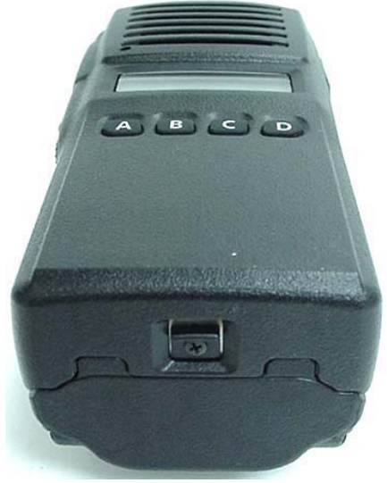
Bottom of DUT with 2000 mAh Li-ion Battery
