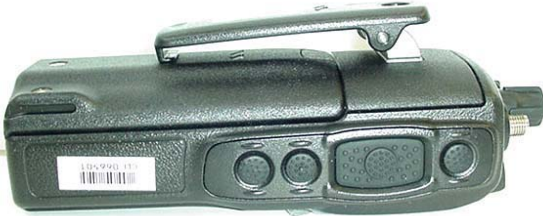
Left Side of DUT with 1150 mAh Li-ion Battery & Belt-Clip
