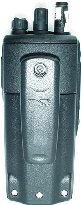
Back of DUT with 1150 mAh Li-ion Battery & Belt-Clip
