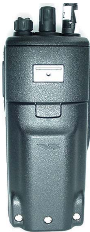
Back of DUT with 2000 mAh Li-ion Battery
