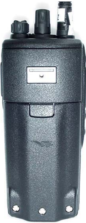
Back of DUT with 1150 mAh Li-ion Battery
