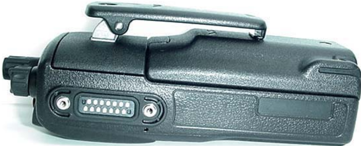
Right Side of DUT with 2000 mAh Li-ion Battery & Belt-Clip
