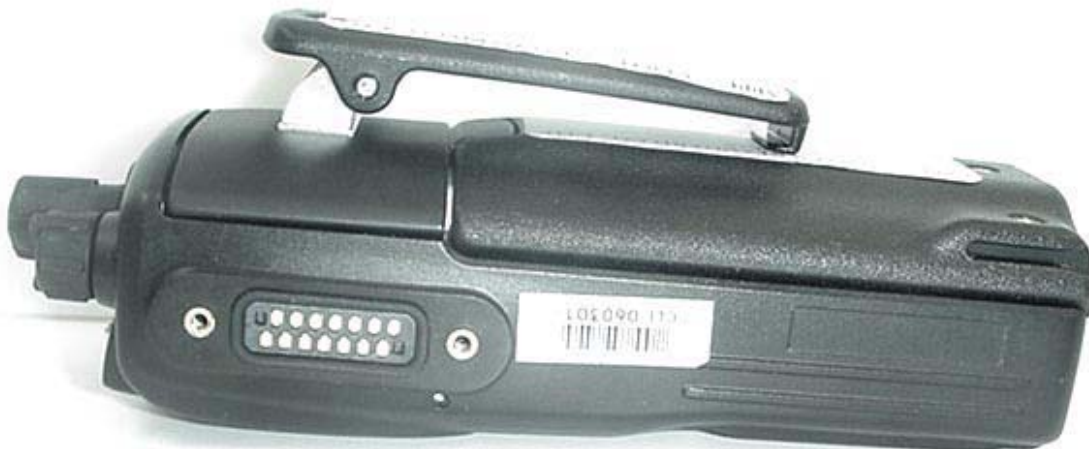
Right Side of DUT with 1150 mAh Li-ion Battery & Belt-Clip
