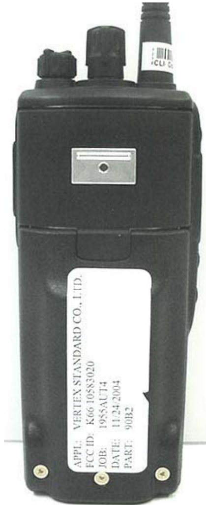
Back of DUT with 2000 mAh Li-ion Battery
