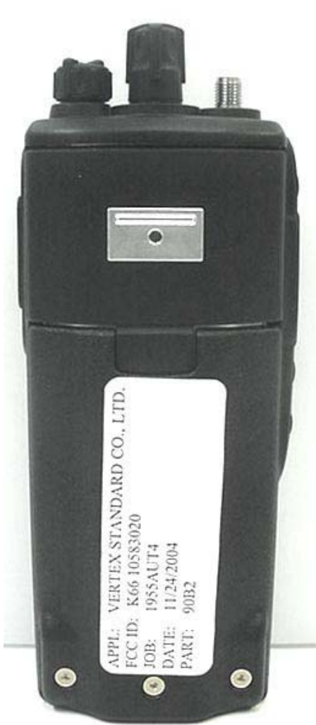
Back of DUT with 1150 mAh Li-ion Battery
