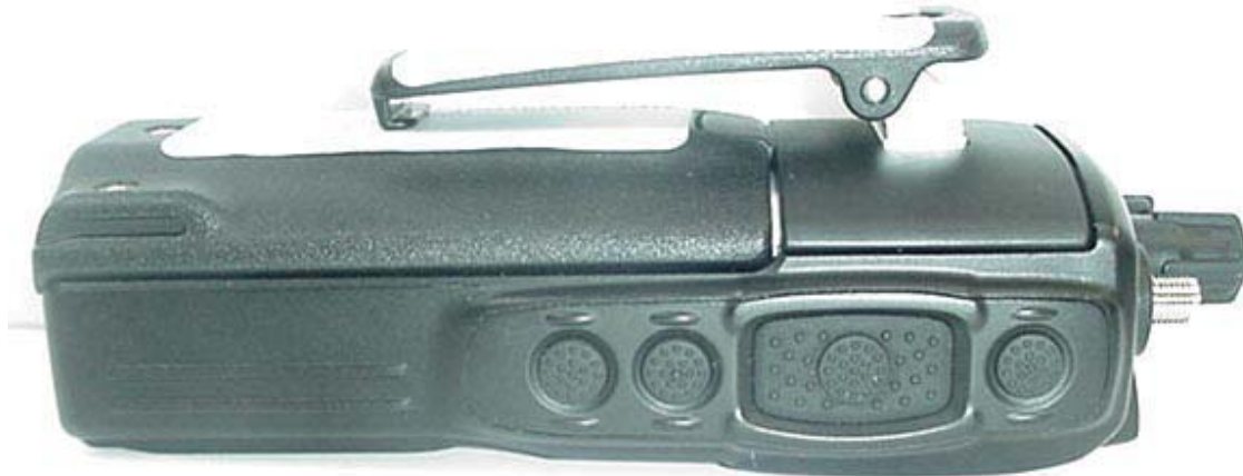
Left Side of DUT with 1150 mAh Li-ion Battery & Belt-Clip
