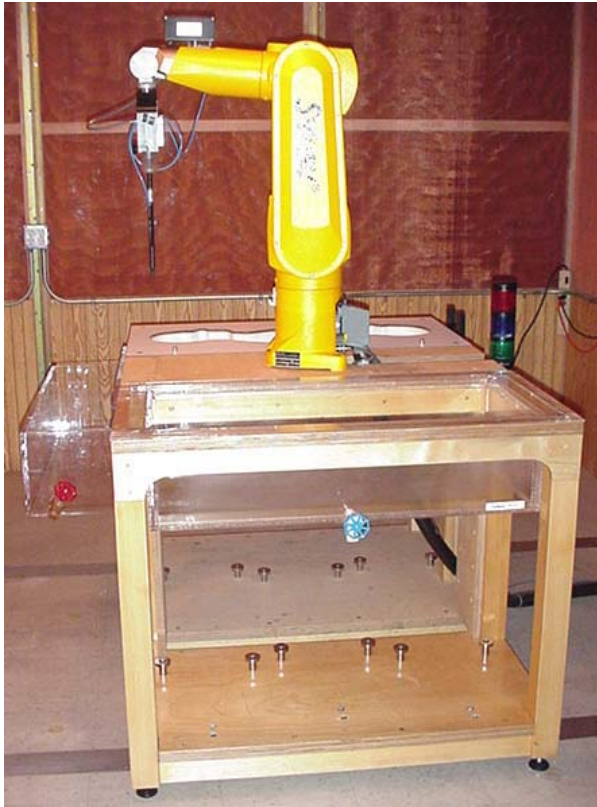
DASY4 SAR Measurement System with validation phantom
