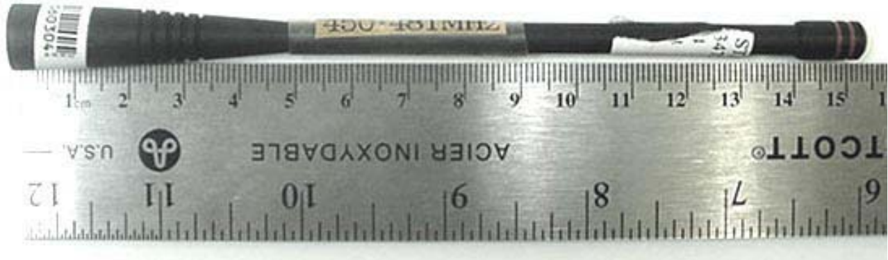
Whip Antenna 450-481 MHz (P/N: ATU-6D)
