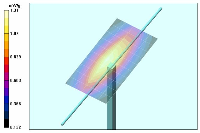
1 g average of 10 measurements: 1.24 mW/g 10 g average of 10 measurements: 0.801 mW/g
