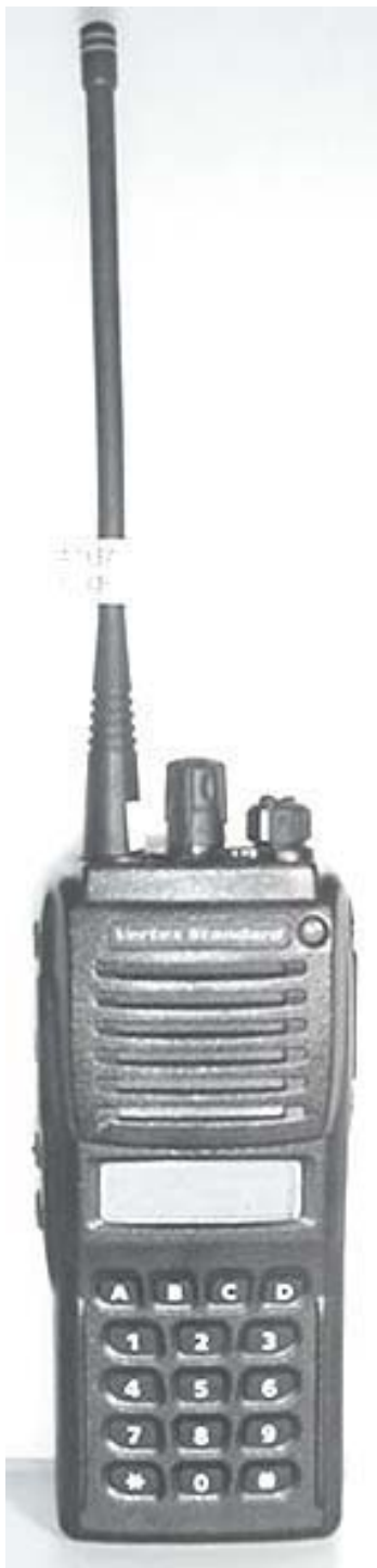
Front of DUT with Whip Antenna (P/N: ATU-6A)
