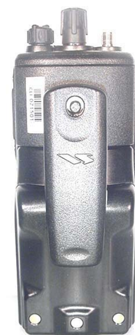
Back of DUT with 3000 mAh Li-ion IS Battery & Belt-Clip
