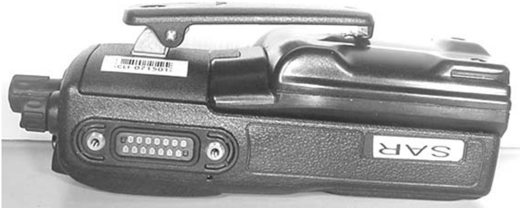
Right Side of DUT with 3000 mAh Li-ion IS Battery & Belt-Clip
