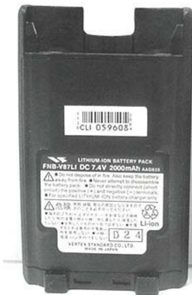
Li-ion Battery 2000 mAh (P/N: FNB-V87LI)
