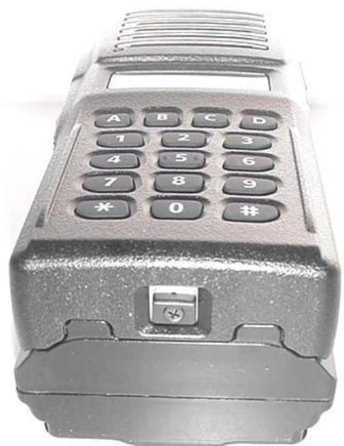
Bottom end of DUT with 3000 mAh Li-ion IS Battery
