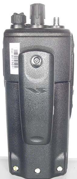
Back of DUT with 1150 mAh Li-ion Battery & Belt-Clip
