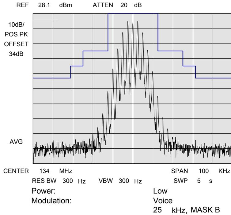
NAME OF TEST: Emission Masks (Occupied Bandwidth)
