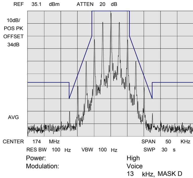
NAME OF TEST: Emission Masks (Occupied Bandwidth)
