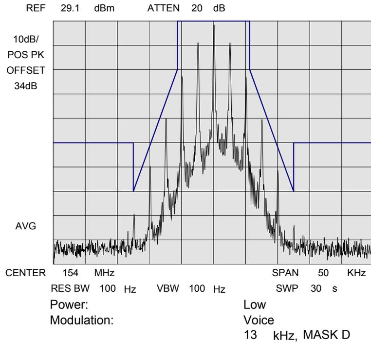
NAME OF TEST: Emission Masks (Occupied Bandwidth)
