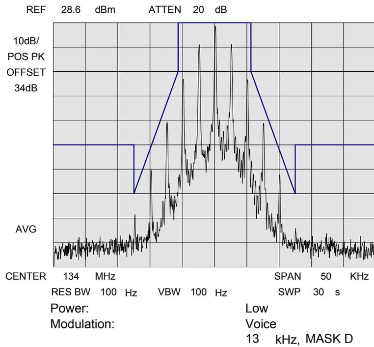
NAME OF TEST: Emission Masks (Occupied Bandwidth)
