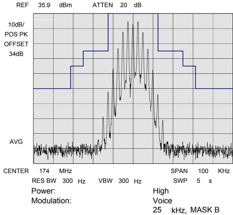
NAME OF TEST: Emission Masks (Occupied Bandwidth)
