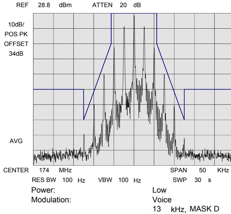
NAME OF TEST: Emission Masks (Occupied Bandwidth)
