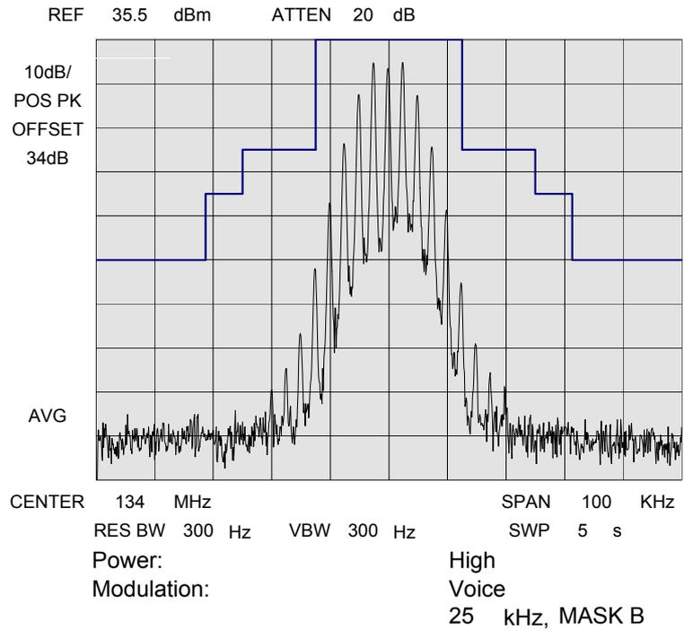
NAME OF TEST: Emission Masks (Occupied Bandwidth)
