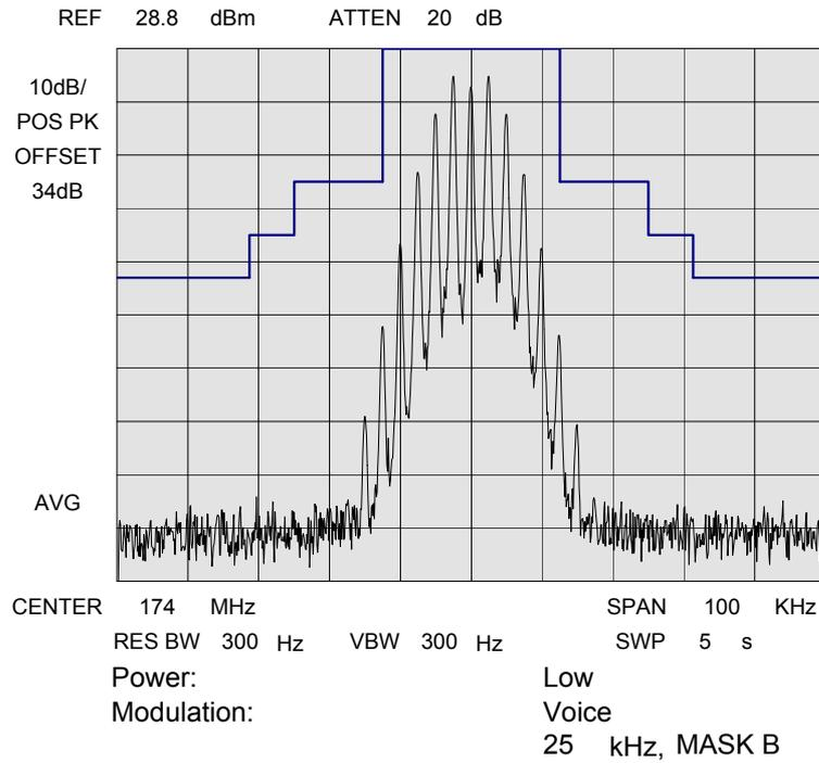
NAME OF TEST: Emission Masks (Occupied Bandwidth)
