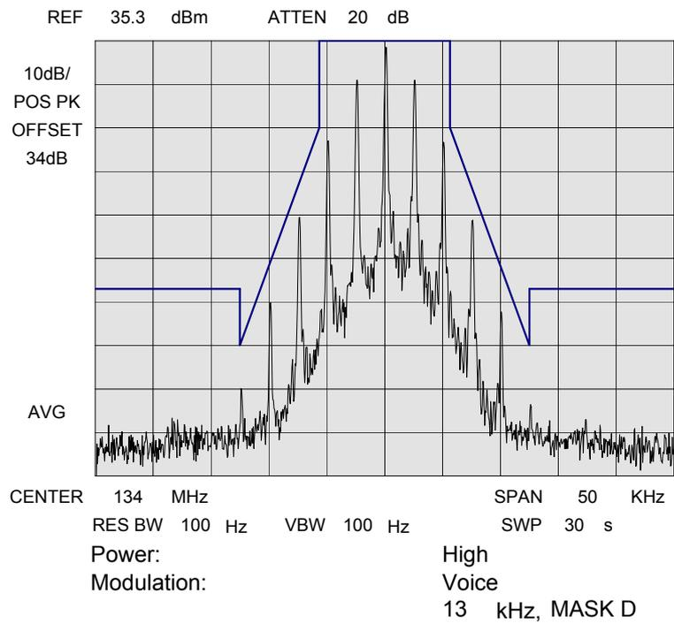
NAME OF TEST: Emission Masks (Occupied Bandwidth)
