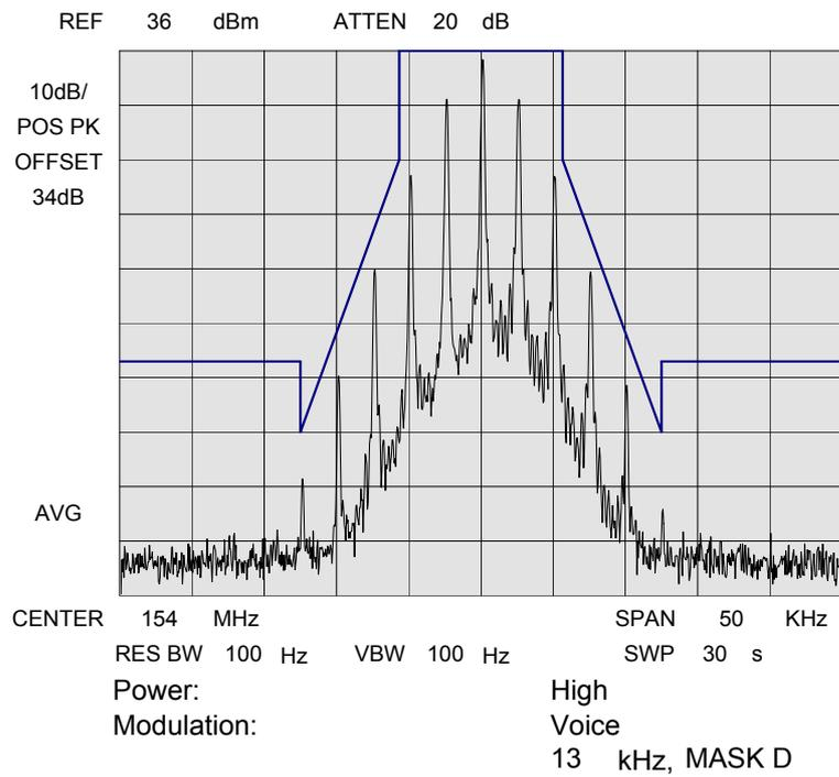
NAME OF TEST: Emission Masks (Occupied Bandwidth)
