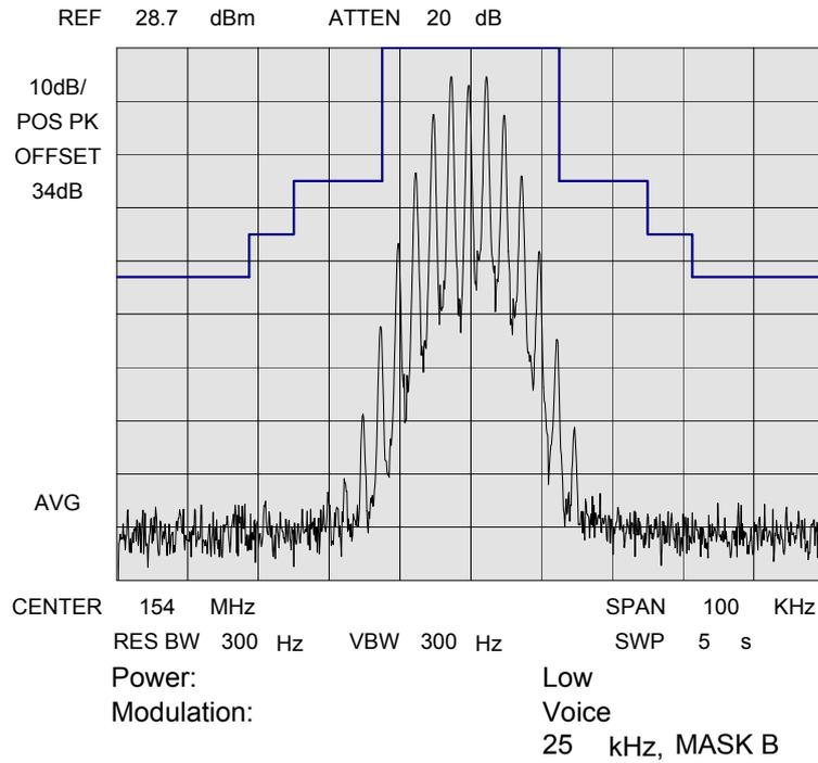
NAME OF TEST: Emission Masks (Occupied Bandwidth)
