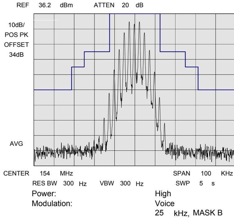
NAME OF TEST: Emission Masks (Occupied Bandwidth)
